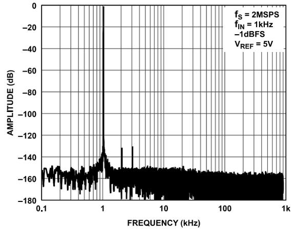
Figure 15. FFT, 2 MSPS,  $f_{IN} = 1$  kHz,  $V_{REF} = 5$  V
