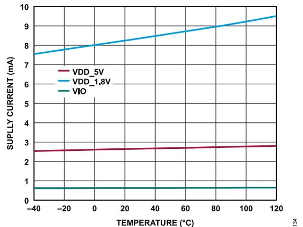
Figure 35. Supply Current vs. Temperature, AD4030-24, 2 MSPS
