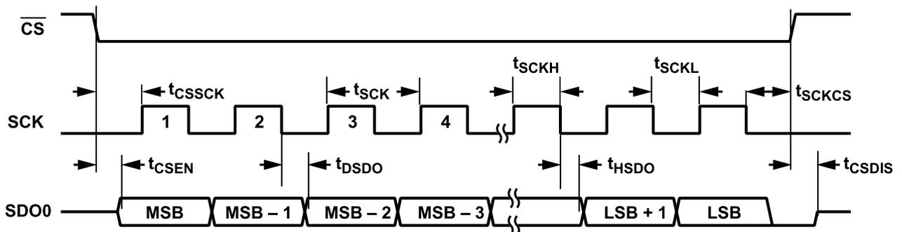
Figure 6. SPI Clocking Mode 1-Lane SDR Timing
