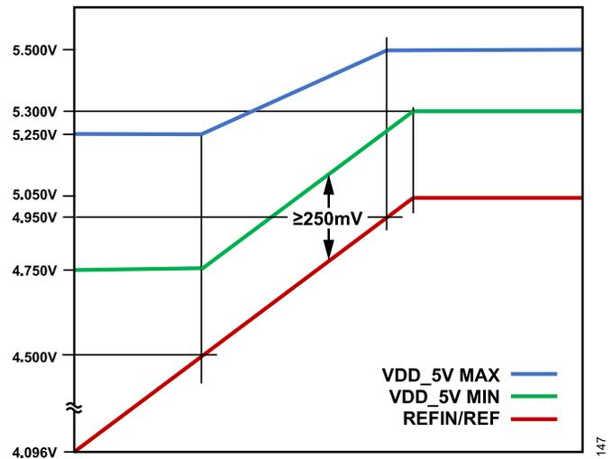
Figure 51. VDD\_5V Minimum and Maximum Values for REFIN/REF
