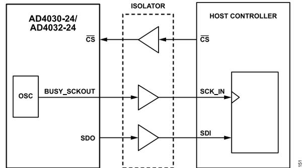
Figure 61. Host Clock Mode Signal Path Example
