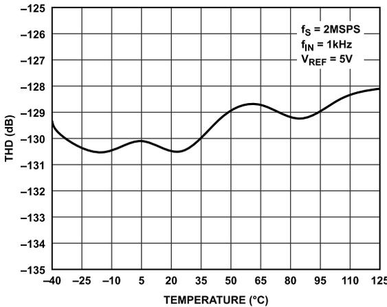
Figure 20. THD vs. Temperature,  $f_{IN} = 1 \text{ kHz}$
