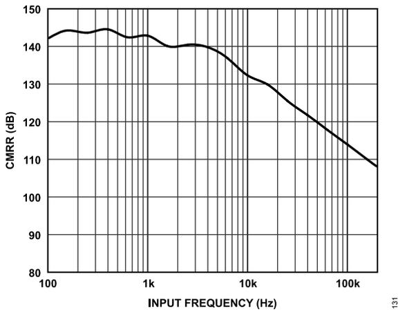
Figure 32. Common-Mode Rejection Ratio (CMRR) vs. Input Frequency
