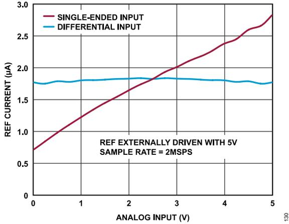
Figure 30. REF Current vs. Analog Input, AD4030-24, 2 MSPS
