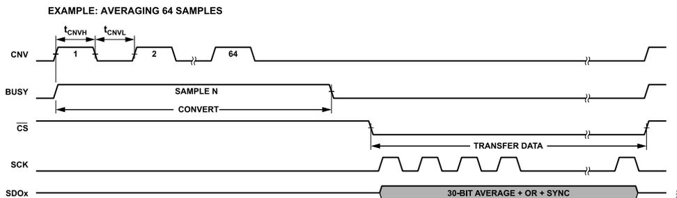
Figure 63. Example Conversion Cycle for Averaging Mode
