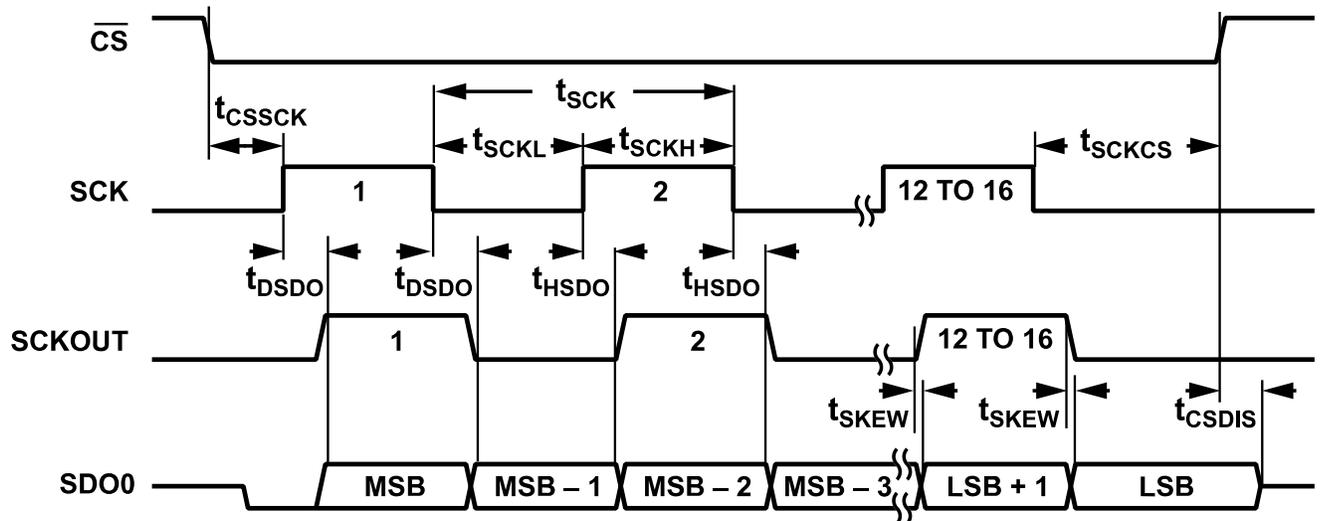
Figure 8. Echo Clock Mode Timing, DDR, 1-Lane
