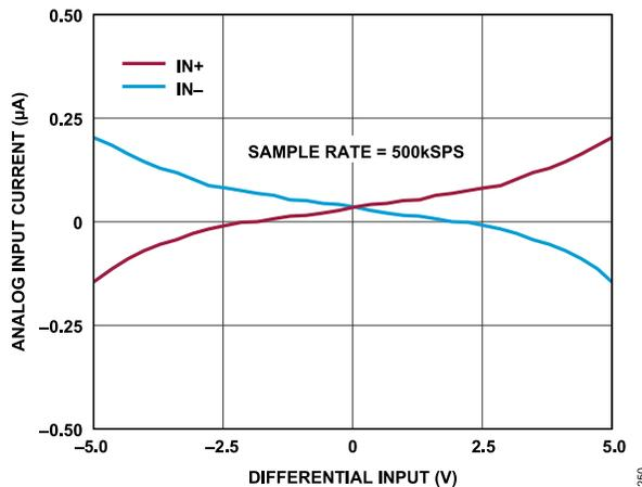
Figure 26. Analog Input Current vs. Differential Input, AD4032-24, 500 kSPS
