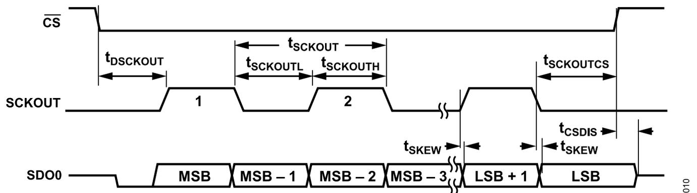
Figure 10. Host Clock Mode Timing, DDR, 1-Lane
