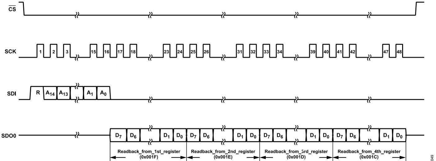
Figure 56. Stream Mode Bulk Register Read Back Operation
