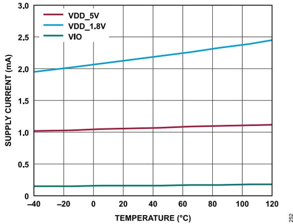
Figure 36. Supply Current vs. Temperature, AD4032-24, 500 kSPS
