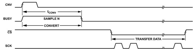
Figure 59. Typical Sample Cycle for SPI Clocking Mode
