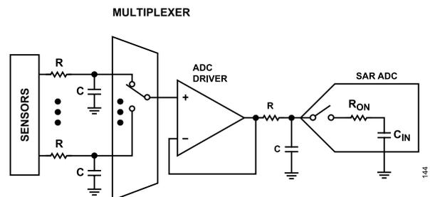
Figure 47. Multiplexed Data Acquisition Signal Using the AD4030-24/AD4032-24
