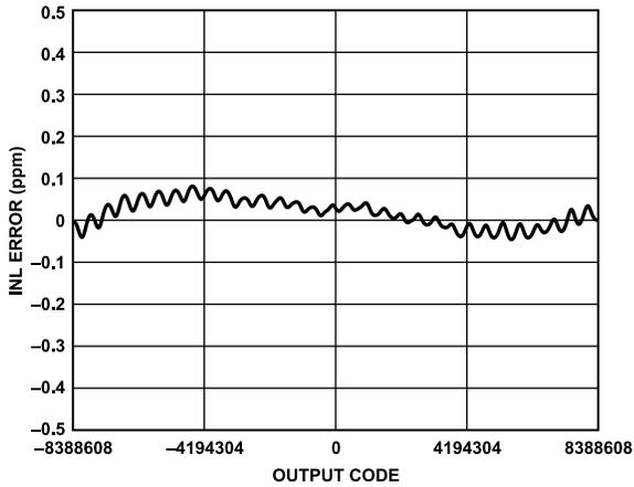
Figure 12. INL Error vs. Output Code, Differential Input
