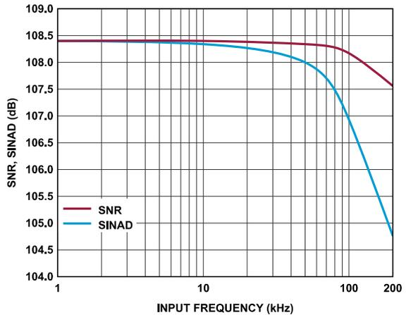
Figure 16. SNR, SINAD vs. Input Frequency
