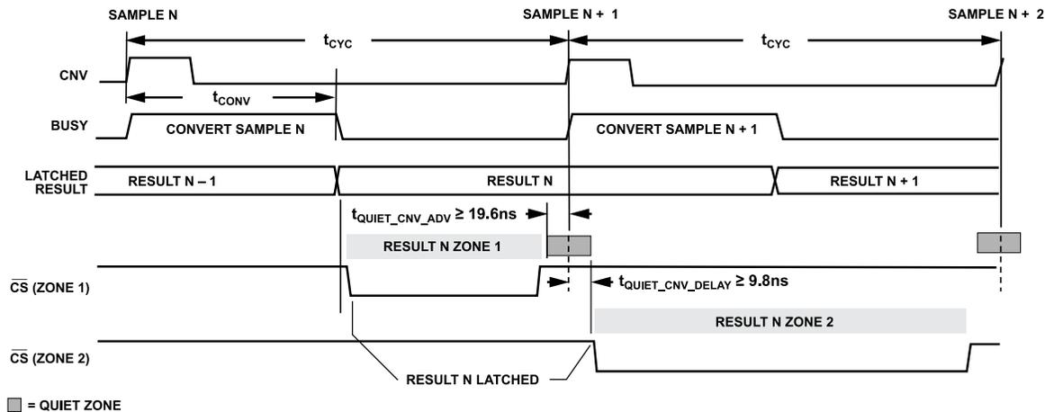
Figure 57. Example Timing for Data Transfer Zones
