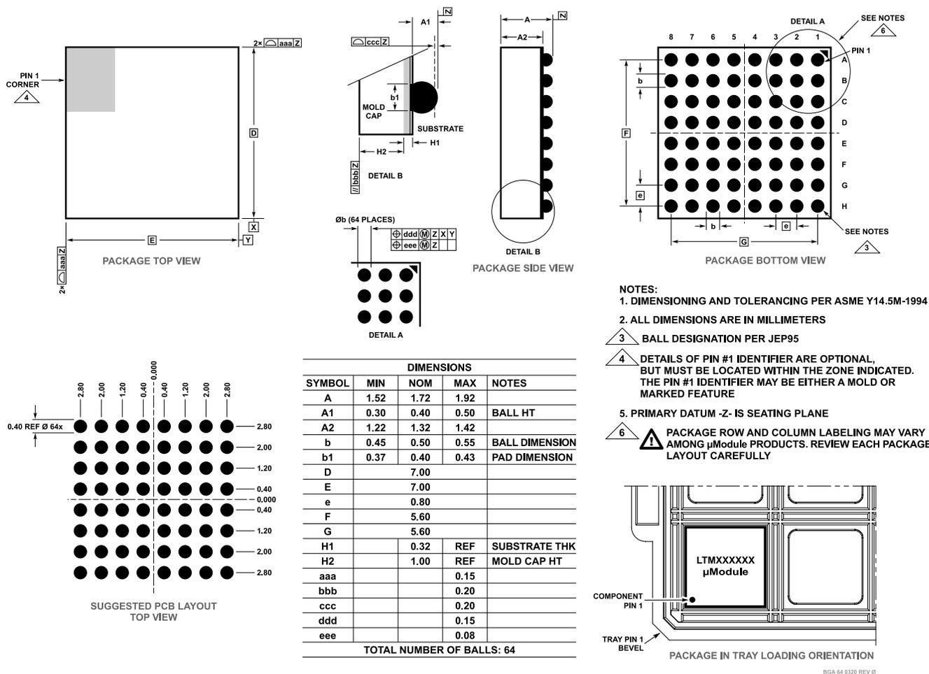
Figure 69. 64-Ball Chip Scale Package Ball Grid Array [CSP\_BGA] (05-08-1797)
