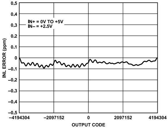
Figure 13. INL Error vs. Output Code, Single-Ended Input
