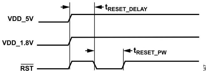
Figure 50. Power-On Reset (POR) Timing
