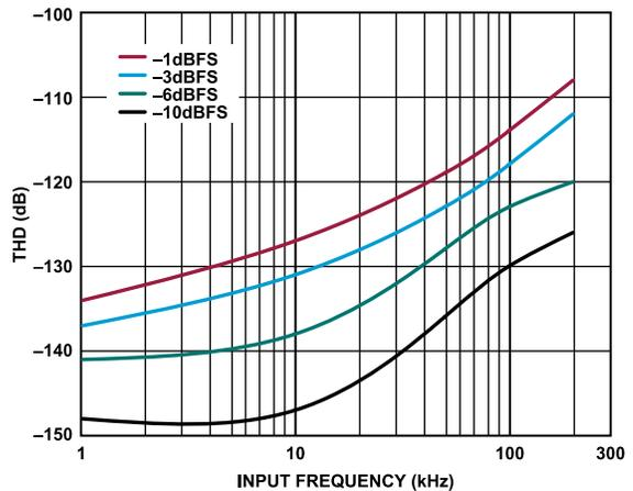
Figure 17. THD vs. Input Frequency, Various Amplitudes
