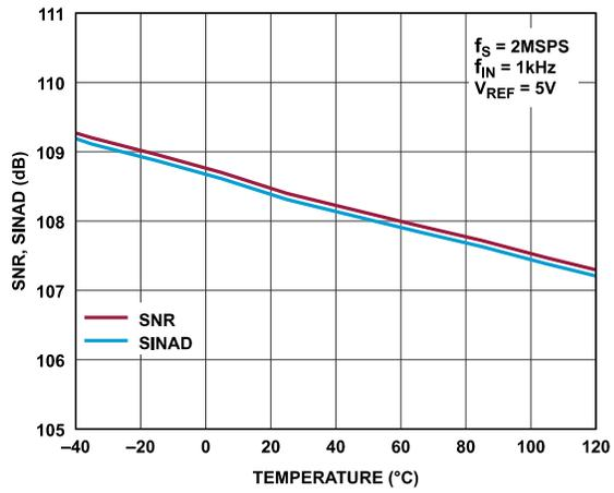
Figure 19. SNR, SINAD vs. Temperature,  $f_{IN} = 1 \text{ kHz}$
