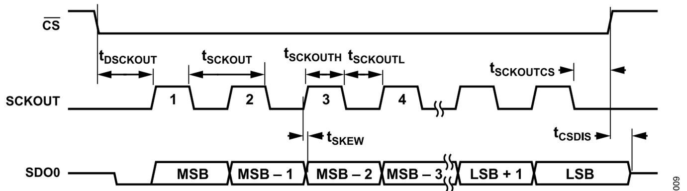
Figure 9. Host Clock Mode Timing, SDR, 1-Lane
