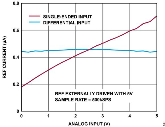
Figure 31. REF Current vs. Analog Input, AD4032-24, 500 kSPS
