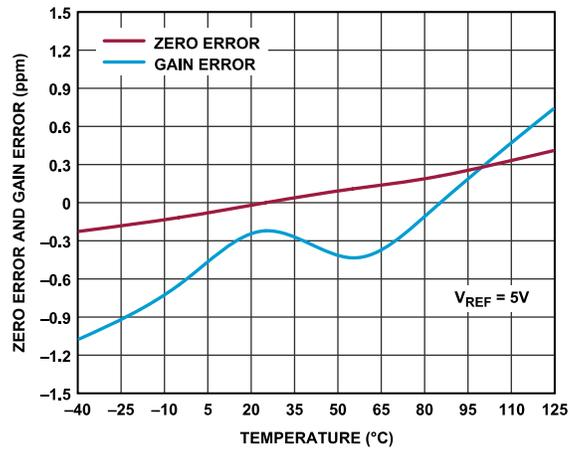
Figure 22. Zero Error and Gain Error vs. Temperature
