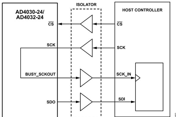
Figure 60. Echo Clock Mode Signal Path Diagram
