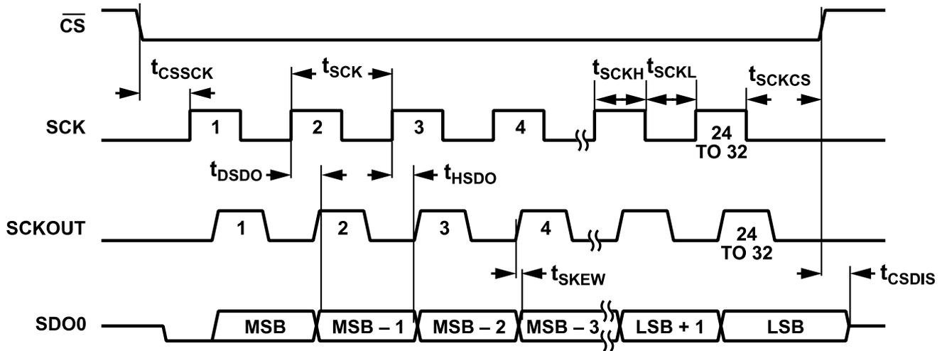
Figure 7. Echo Clock Mode Timing, SDR, 1-Lane
