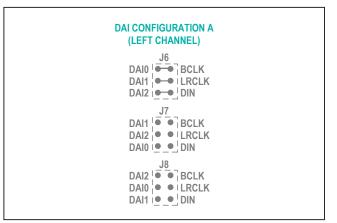
Figure 3. DAI Configuration A (Left-Channel for I<sup>2</sup>S/Left-Justified Operation)
