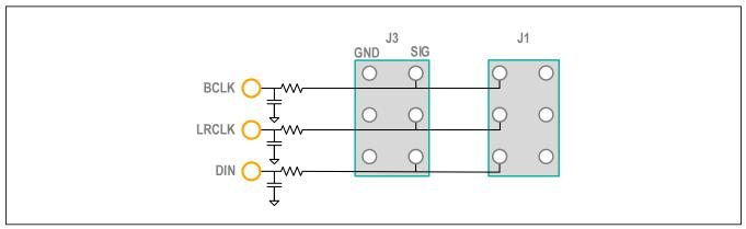
Figure 4. MAX98361 DAI Interface Headers (PCM)
