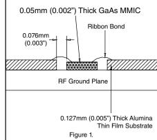
Cleanliness: Handle the chips in a clean environment. DO NOT attempt to clean the chip using liquid cleaning systems.
