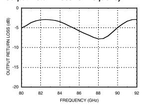
Note: Measured Performance Characteristics (Typical Performance at 25°C) Vdd1 = Vdd2 = 4V, Idd1 = 80mA, Idd2 = 80mA
