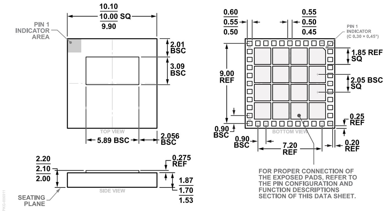
Figure 27. 40-Terminal Land Grid Array Package [LGA] (CC-40-12)
