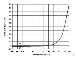
Figure 42. Operational Amplifier Bias Current vs. Temperature
