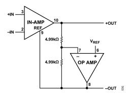
Figure 53. Differential Output Using Operational Amplifier
