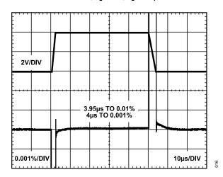
Figure 28. Instrumentation Amplifier Large Signal Pulse Response, G = 1,  $V_S = 5$  V
