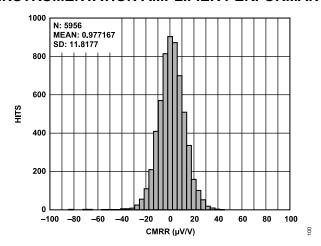
Figure 3. Instrumentation Amplifier CMR Distribution, G = 1
