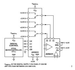
Figure 55. Converting Single-Supply Control Signals to Dual Supply
