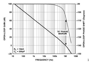
Figure 35. Operational Amplifier Open-Loop Gain and Phase vs. Frequency,  $V_0 = 5 V$
