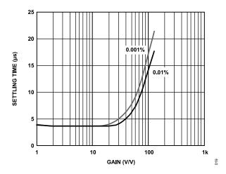
Figure 31. Instrumentation Amplifier Settling Time vs. Gain for a 4 V p-p Step,  $V_S = 5 \text{ V}$
