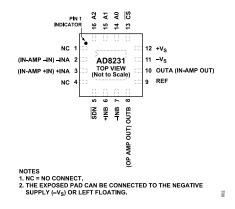
Figure 2. Pin Configuration
