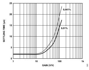
Figure 32. Instrumentation Amplifier Settling Time vs. Gain for a 2 V p-p Step,  $V_S = 3 V$
