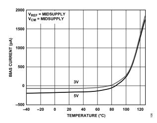
Figure 9. Instrumentation Amplifier Bias Current vs. Temperature
