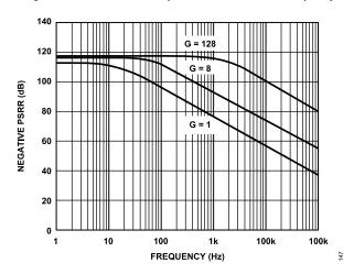
Figure 20. Instrumentation Amplifier Negative PSRR vs. Frequency
