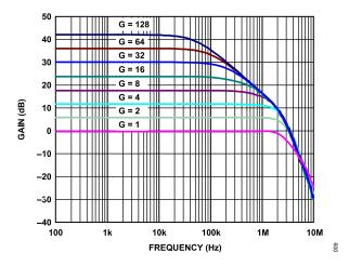
Figure 15. Instrumentation Amplifier Gain vs. Frequency
