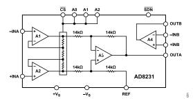
Figure 49. Simplified Schematic
