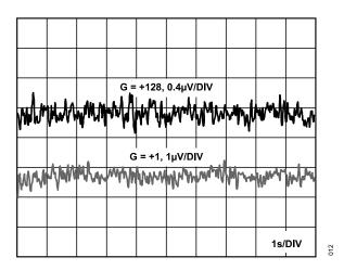
Figure 21. Instrumentation Amplifier 0.1 Hz to 10 Hz Noise
