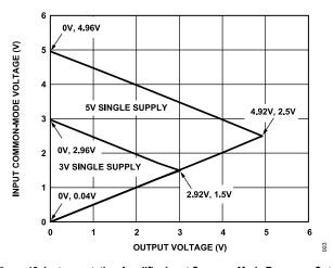
Figure 12. Instrumentation Amplifier Input Common-Mode Range vs. Output Voltage, All Gains,  $V_{REF} = 0 \text{ V}$
