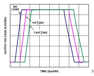
Figure 40. Operational Amplifier Large Signal Transient Response, V<sub>S</sub> = 3 V
