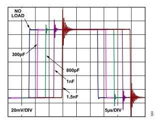
Figure 38. Operational Amplifier Small Signal Response for Various Capacitive Loads,  $V_S = 3 V$
