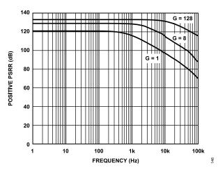
Figure 19. Instrumentation Amplifier Positive PSRR vs. Frequency
