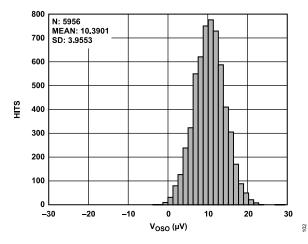
Figure 5. Instrumentation Amplifier Output Offset Voltage Distribution
