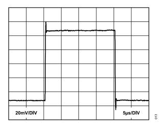
Figure 25. Instrumentation Amplifier Small Signal Pulse Response, G = 1,  $R_L$ = 2  $k\Omega$ ,  $C_L$  = 500 pF
