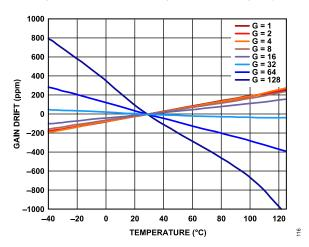
Figure 16. Instrumentation Amplifier Gain Drift vs. Temperature
