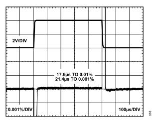
Figure 30. Instrumentation Amplifier Large Signal Pulse Response, G = 128,  $V_S = 5 V$
