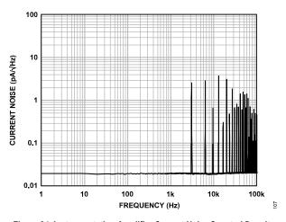
Figure 24. Instrumentation Amplifier Current Noise Spectral Density
