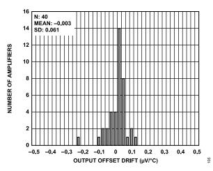
Figure 8. Instrumentation Amplifier Output Offset Drift, -40°C to +125°C
