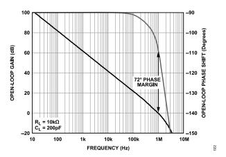
Figure 36. Operational Amplifier Open-Loop Gain and Phase vs. Frequency,
