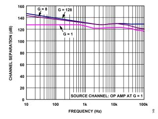
Figure 48. Channel Separation vs. Frequency
