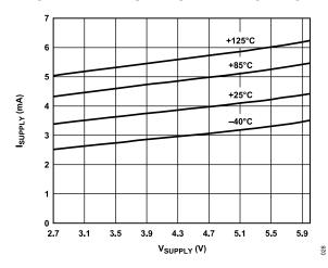
Figure 47. Supply Current vs. Supply Voltage
