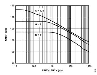
Figure 17. Instrumentation Amplifier CMRR vs. Frequency
