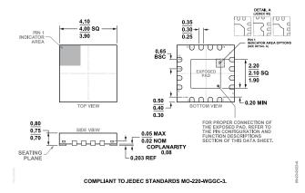
Figure 57. 16-Lead Lead Frame Chip Scale Package [LFCSP]
