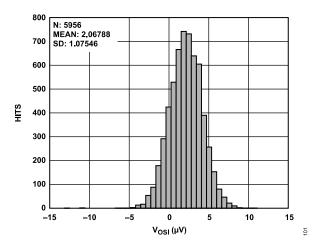
Figure 4. Instrumentation Amplifier Input Offset Voltage Distribution
