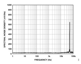
Figure 41. Operational Amplifier Voltage Spectral Noise Density vs. Frequency
