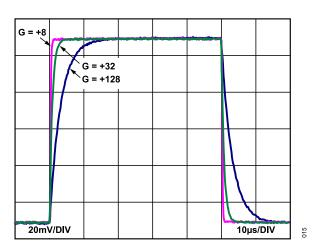
Figure 27. Instrumentation Amplifier Small Signal Pulse Response, G = 8, 32, and 128,  $R_L$  = 2  $k\Omega$ ,  $C_L$  = 500 pF
