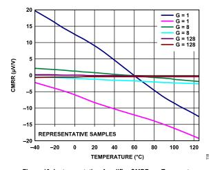
Figure 18. Instrumentation Amplifier CMRR vs. Temperature
