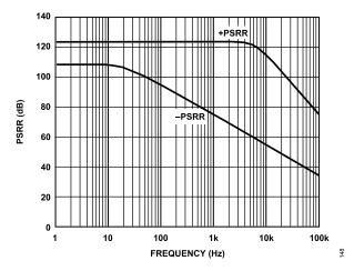
Figure 46. Operational Amplifier Power Supply Rejection Ratio
