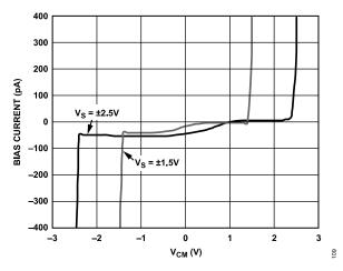
Figure 43. Operational Amplifier Bias Current vs. Common Mode
