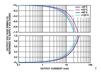
Figure 45. Operational Amplifier Output Voltage Swing vs. Output Current,  $V_S$ = 5 V
