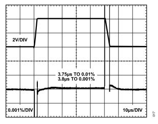
Figure 29. Instrumentation Amplifier Large Signal Pulse Response, G = 8,  $V_S = 5$  V
