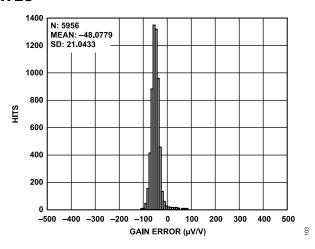
Figure 6. Instrumentation Amplifier Gain Distribution, G = 1
