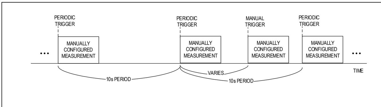
Figure 5. Moisture Detection Triggering for Manual Configuration
