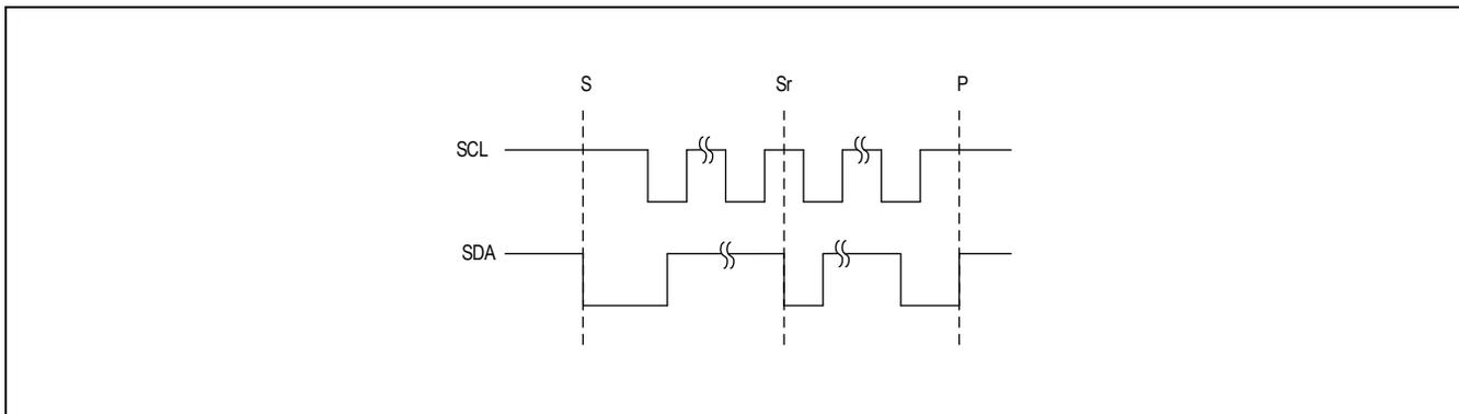
Figure 10. I<sup>2</sup>C START, STOP, and REPEATED START Conditions
