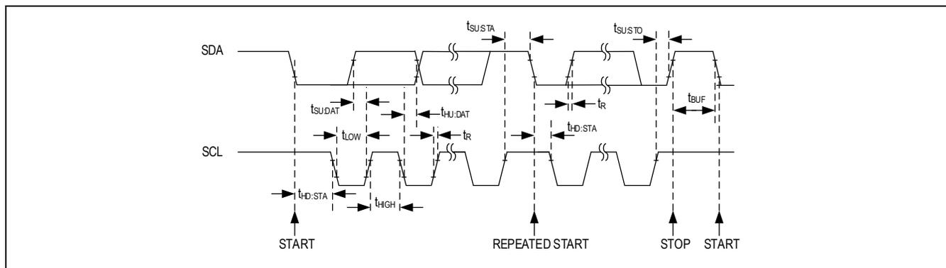
Figure 9. I<sup>2</sup>C Interface Timing
