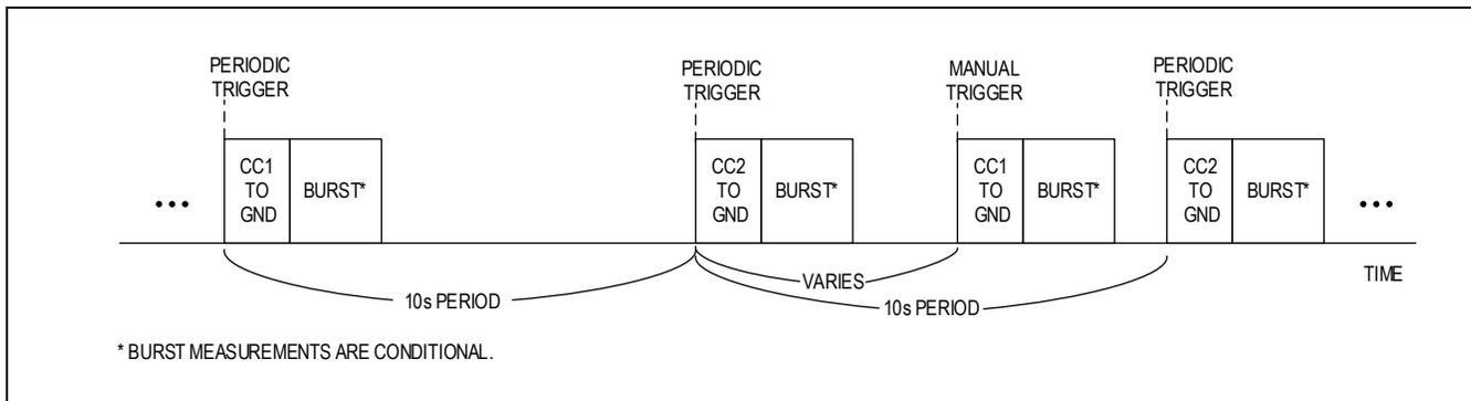
Figure 4. Moisture Detection Triggering for Automatic Configuration
