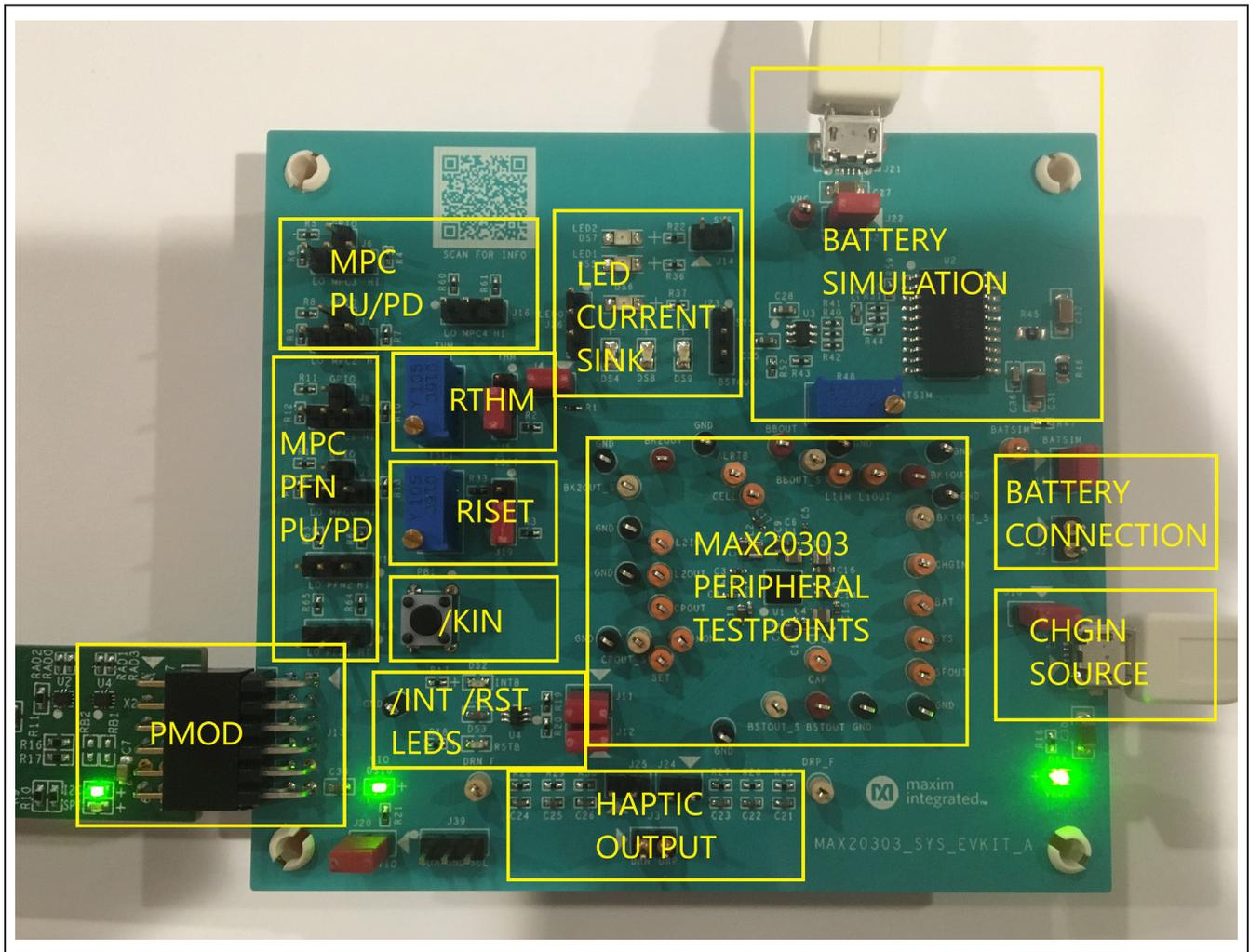
Figure 16. MAX20303 EVSYSKIT Block Annotated Picture
