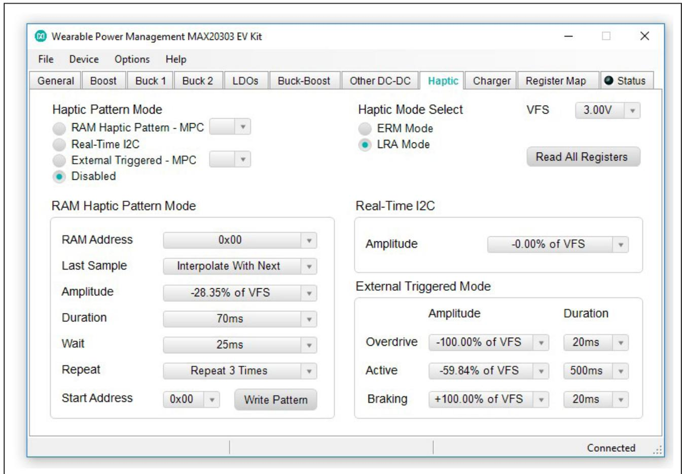
Figure 11. Haptic Tab
