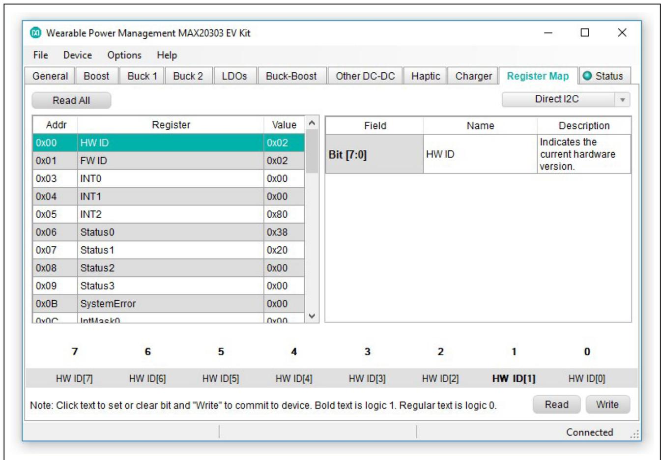
Figure 13. Register Map Tab Direct I<sup>2</sup>C
