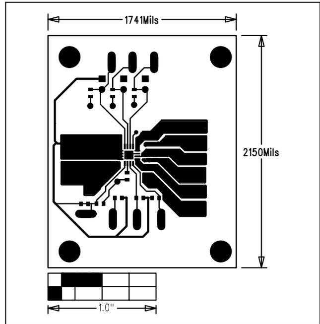
Figure 3. MAX1564 EV Kit PC Board Layout—Component Side
