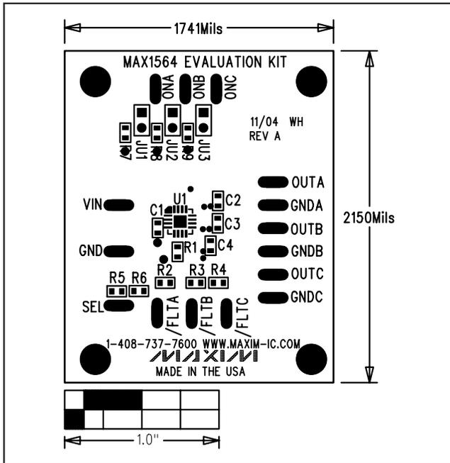
Figure 2. MAX1564 EV Kit Component Placement Guide—Top Silkscreen
