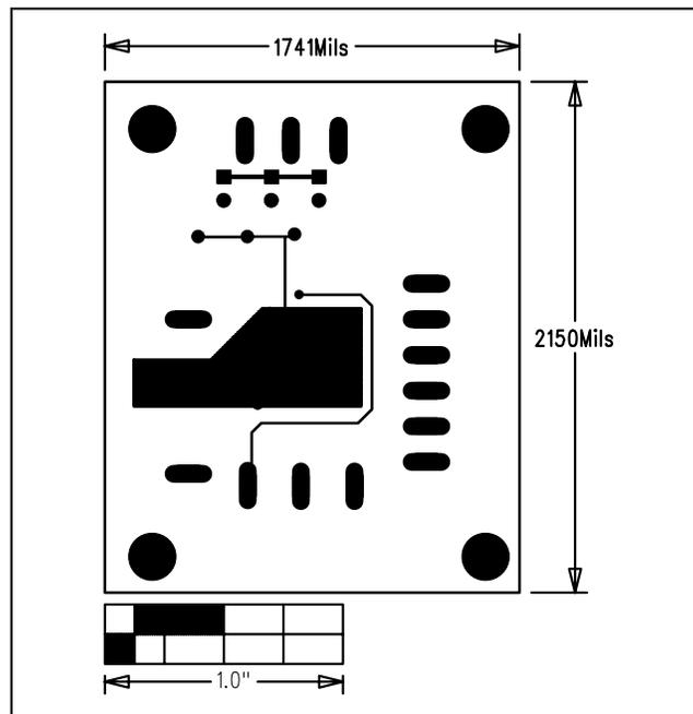
Figure 4. MAX1564 EV Kit PC Board Layout—Solder Side
