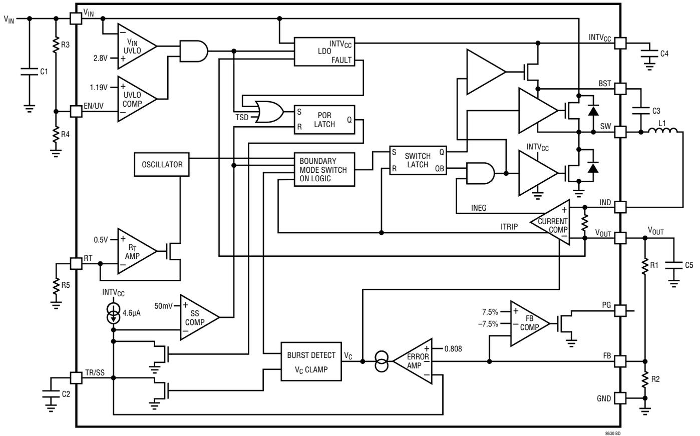
Figure 1. Block Diagram
