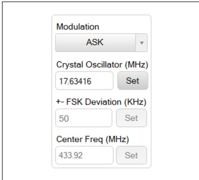
Figure 26. Setting of Modulation and Frequencies
