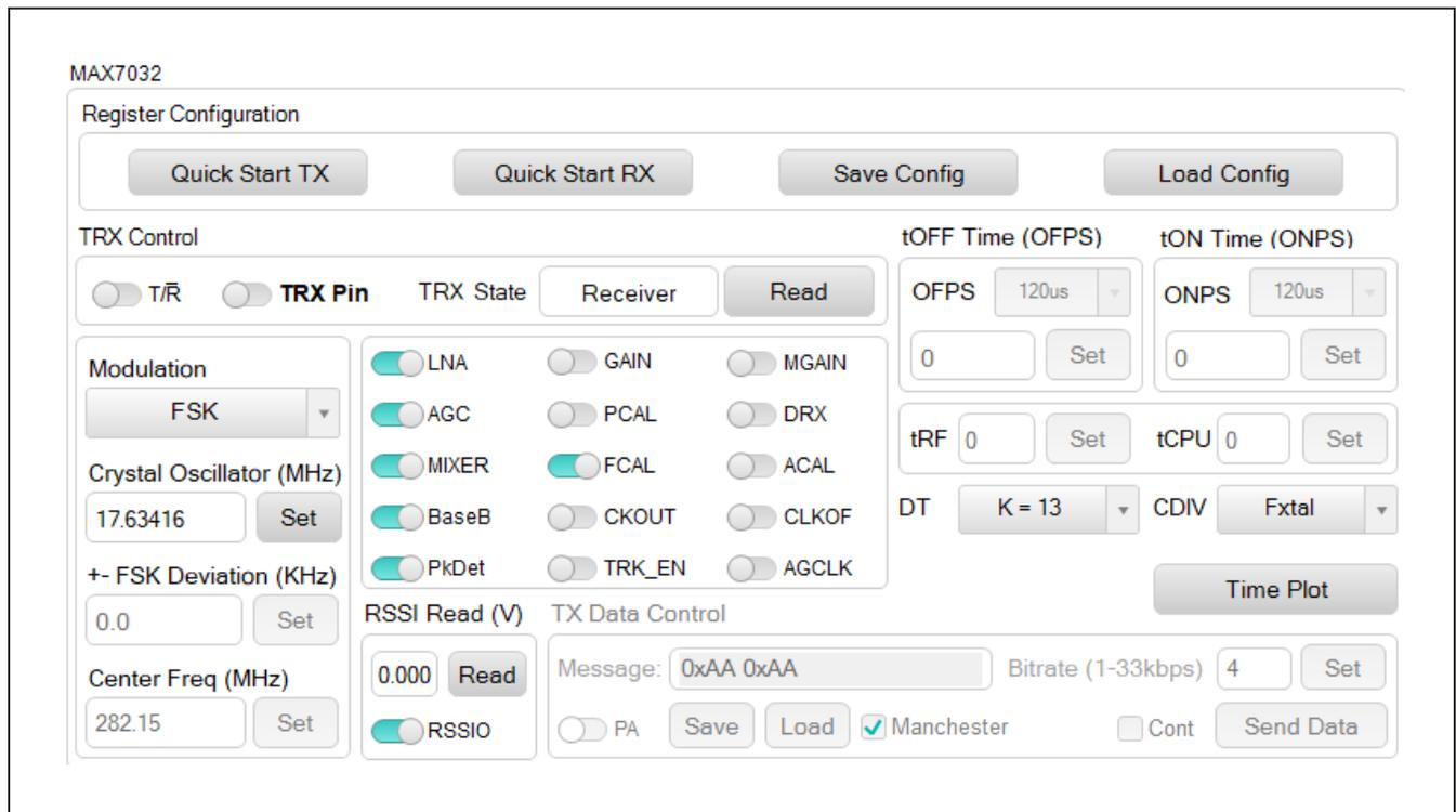
Figure 15. Device Settings for FSK Receiver
