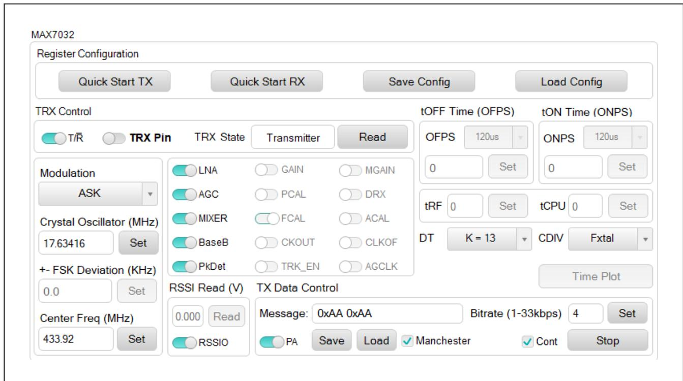
Figure 17. Device Settings for ASK Transmitter
