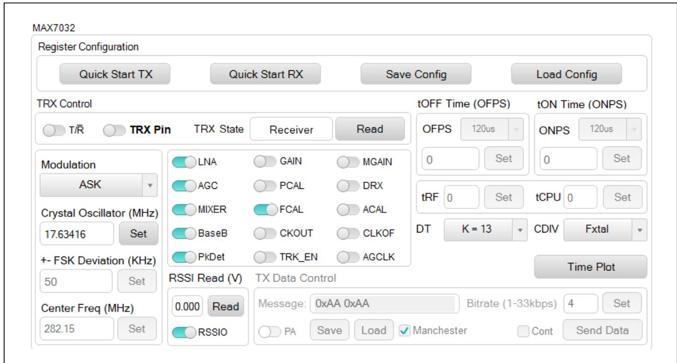
Figure 14. Device Settings for ASK Receiver
