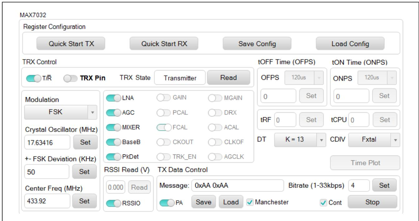
Figure 18. Device Settings for FSK Transmitter
