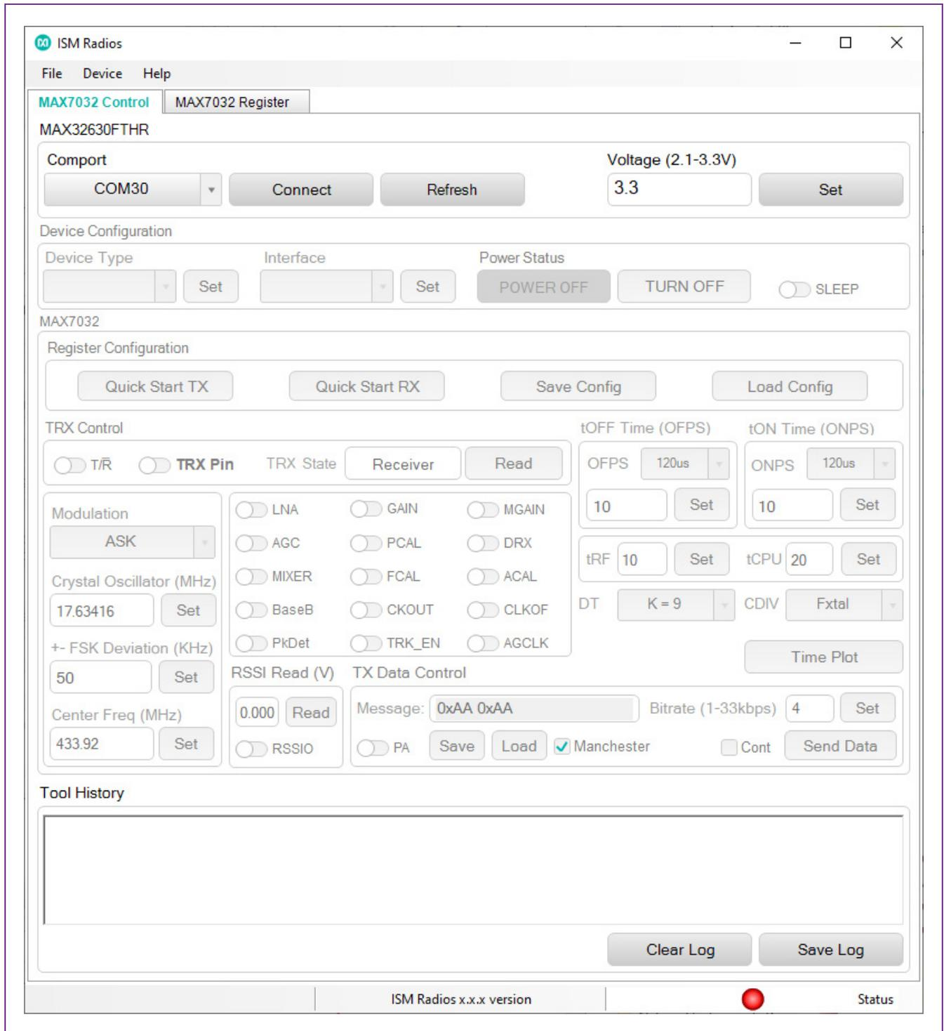
Figure 6. ISM Radios GUI Software Startup
