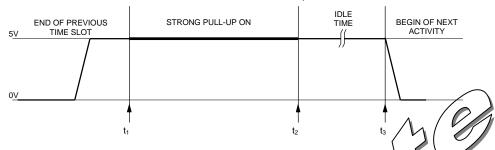
The minimum duration of a strong pull-up of infinite duration strongly depends on the band rate of the communication between host and DS2480. The host must first receive the response byte of the single-bit command, react to it and then transmit the termination command. Neglecting the hosts response time, the shortest duration of an infinite strong pull-up therefore is 13.6 µs at 115.2 kbps, 347.2 µs at 57.6 kbps, 1.04 ms at 19.2 kbps and 2.08 ms at 9.6 kbps.
