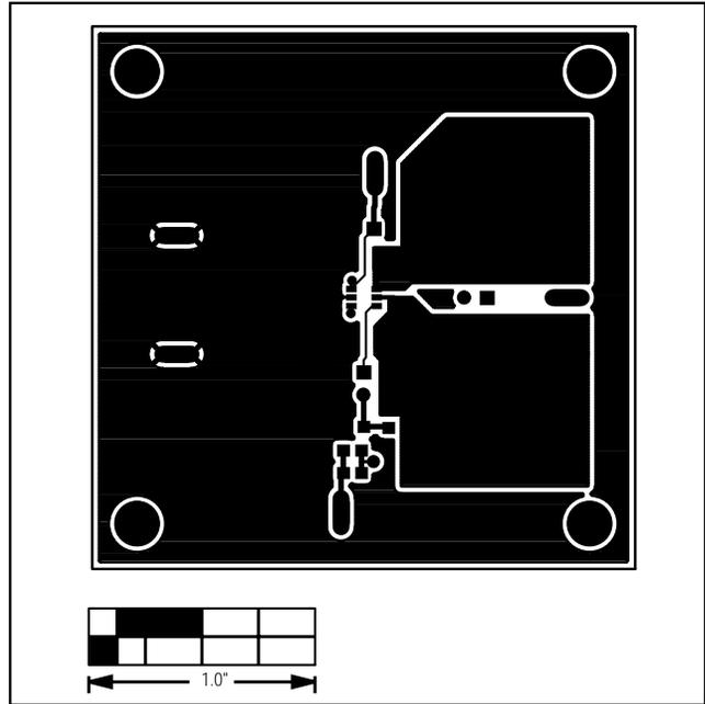
Figure 3. MAX1982 EV Kit PC Board Layout—Component Side
