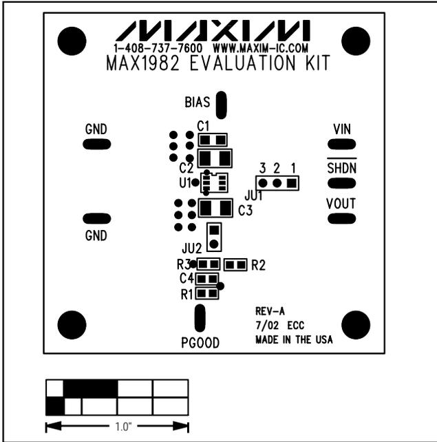
Figure 2. MAX1982 EV Kit Component Placement Guide—Component Side
