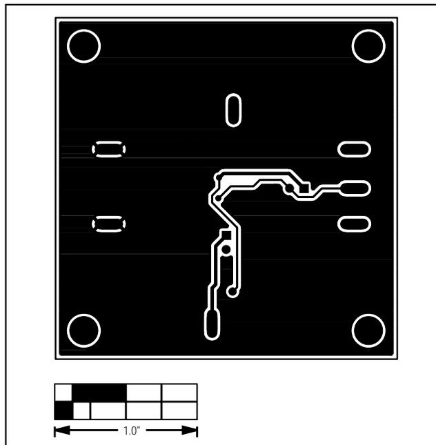
Figure 4. MAX1982 EV Kit PC Board Layout—Solder Side
