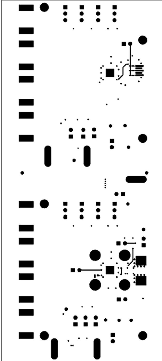
Figure 9. MAX3865 EV Kit PC Board Layout—Solder Side
