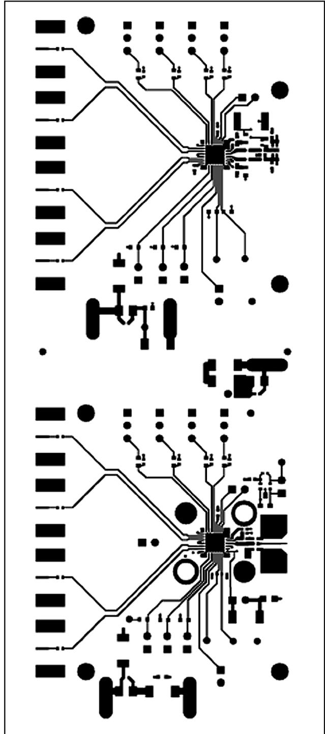
Figure 6. MAX3865 EV Kit PC Board Layout—Component Side
