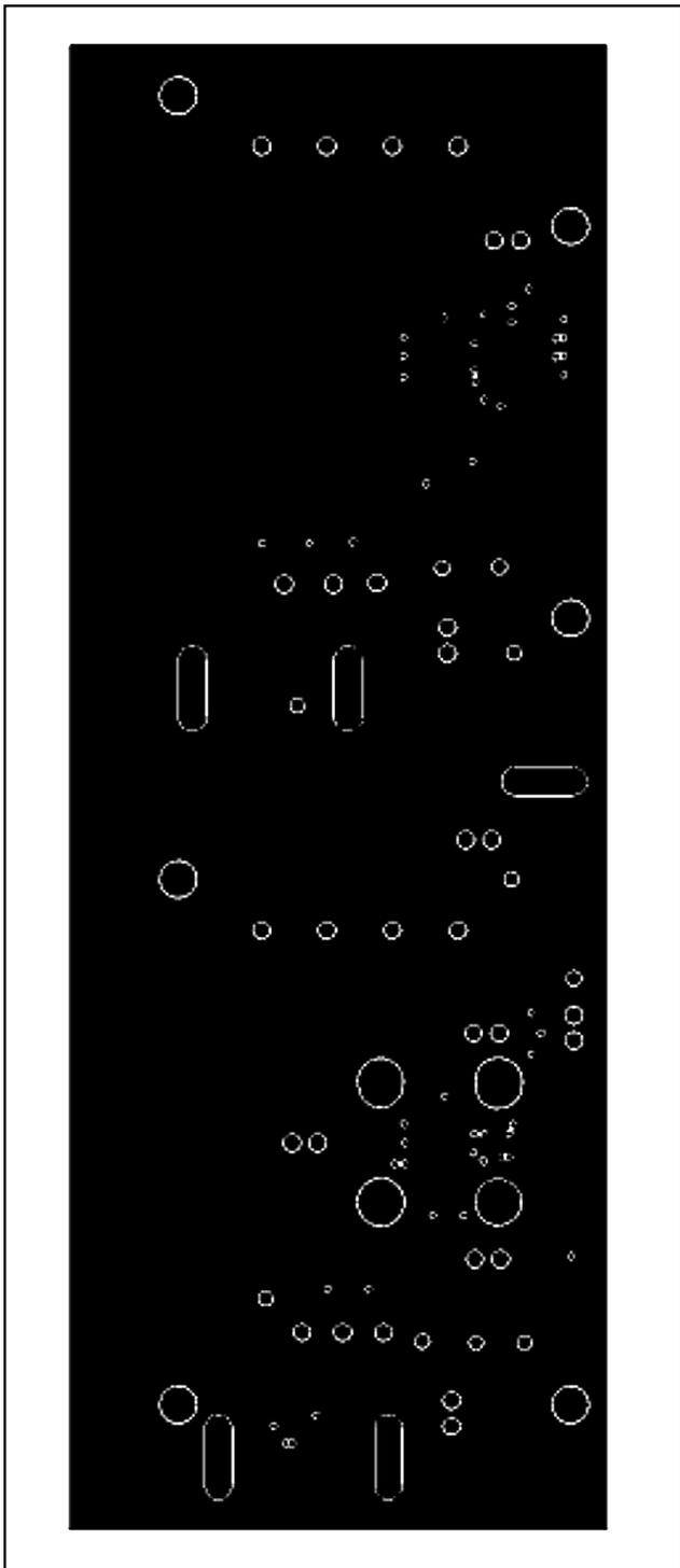
Figure 7. MAX3865 EV Kit PC Board Layout—Ground Plane
