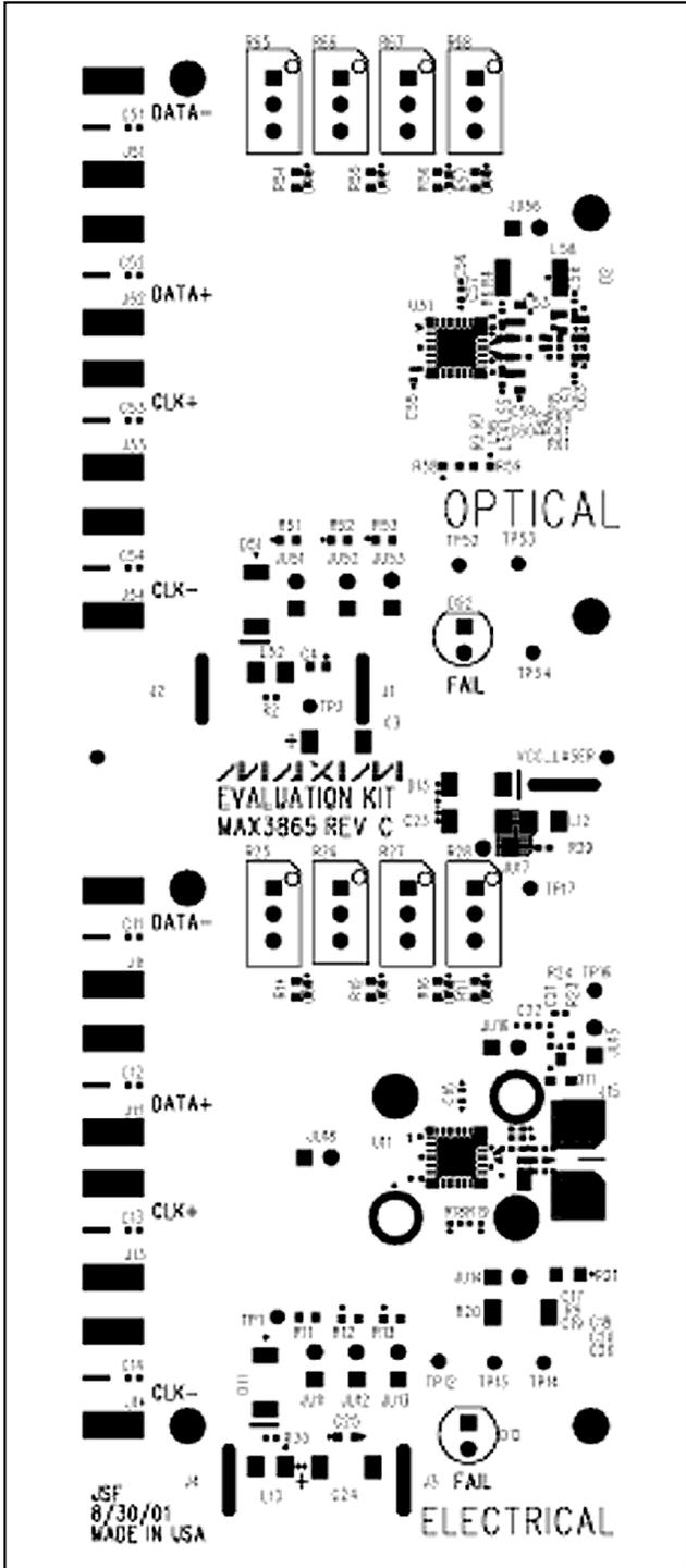
Figure 5. MAX3865 EV Kit Component Placement Guide—Component Side
