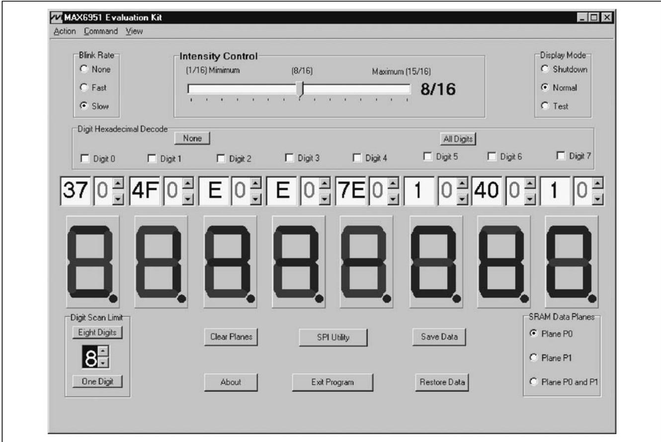
Figure 1. Main Panel for MAX6951 EV Kit
