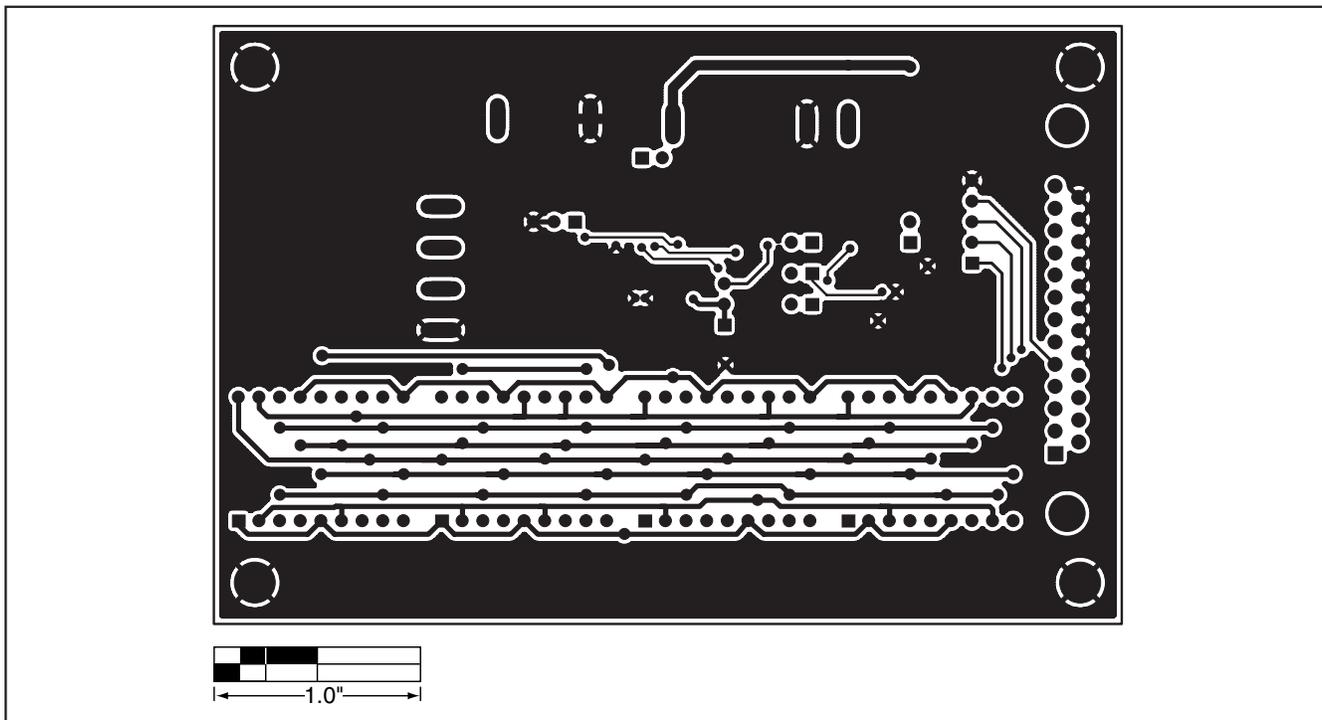
Figure 8. MAX6951 EV Kit PCB Layout—Solder Side
