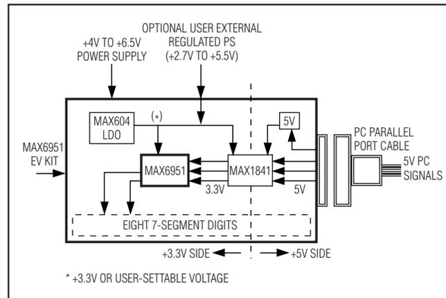
Figure 3. MAX6951 EV Kit Level-Translation Functional Diagram
