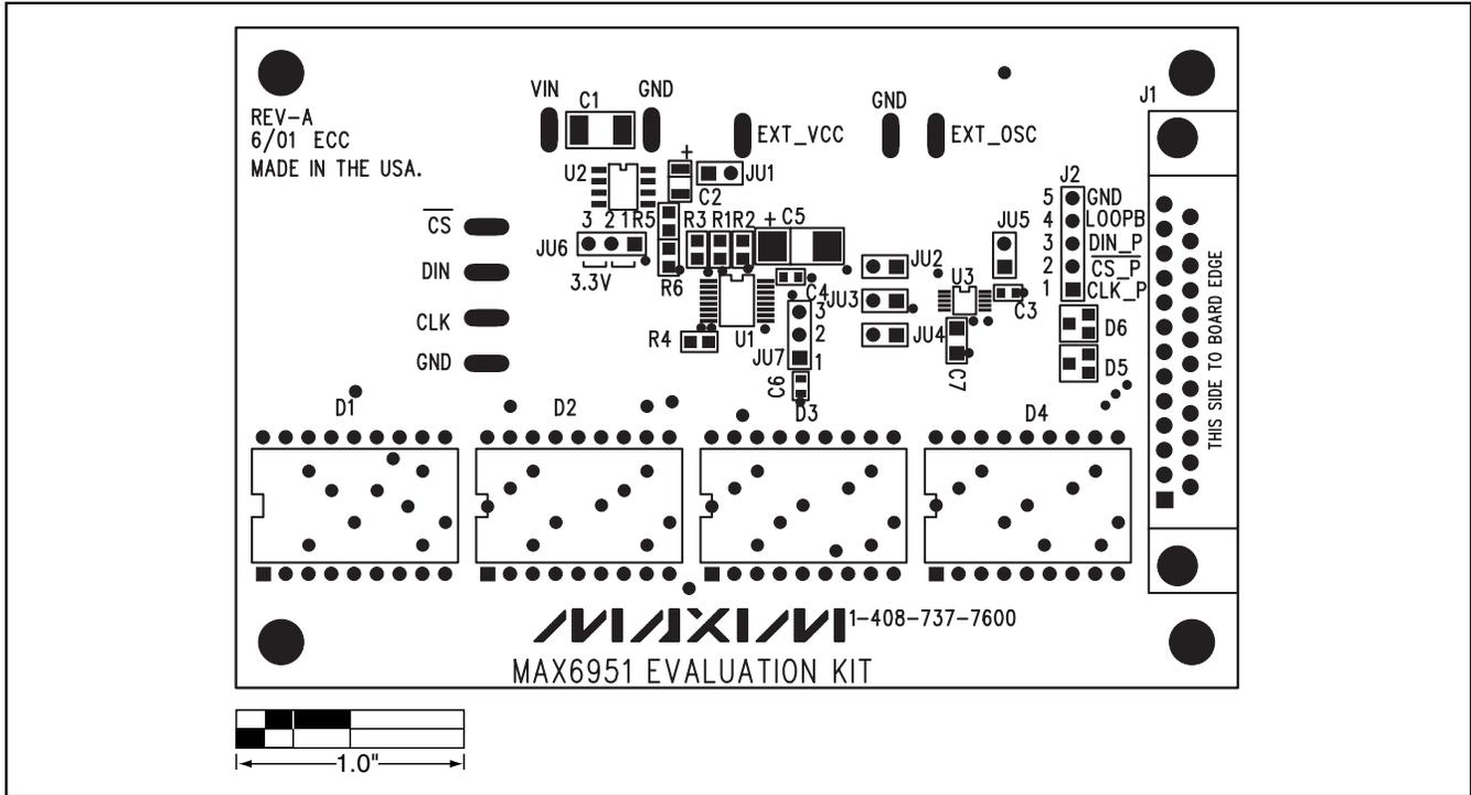
Figure 6. MAX6951 EV Kit Component Placement Guide—Component Side
