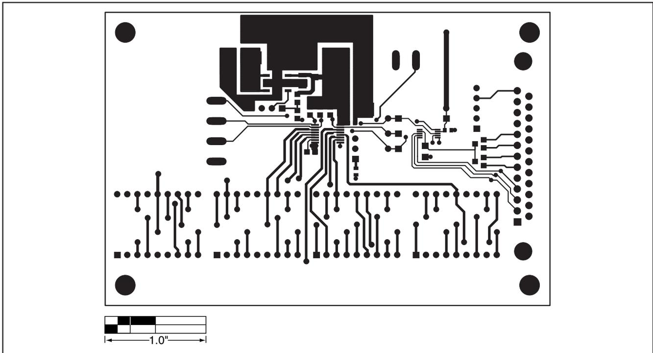
Figure 7. MAX6951 EV Kit PCB Layout—Component Side
