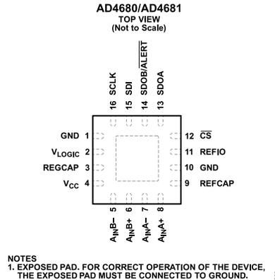
Figure 6. Pin Configuration
