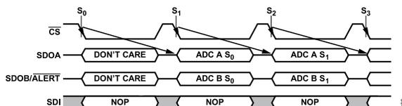
Figure 38. Reading Conversion Results for 2-Wire Mode
