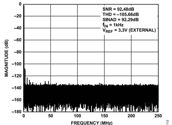
Figure 11. AD4681 FFT,  $V_{REF} = 3.3\text{ V}$  External
