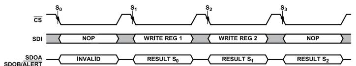
Figure 42. Register Write
