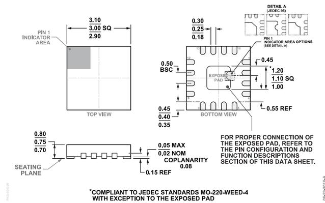
Figure 44. 16-Lead Lead Frame Chip Scale Package [LFCSP]
