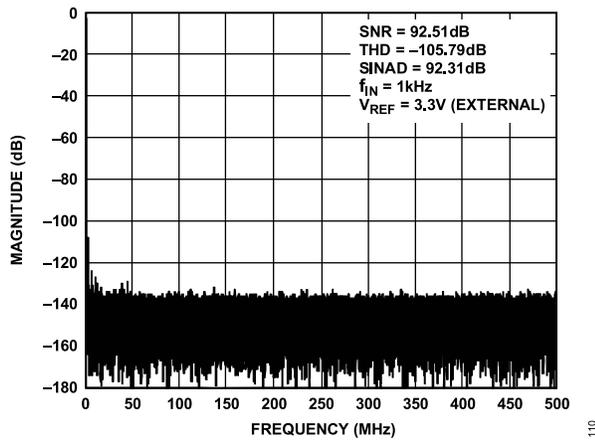
Figure 8. AD4680 FFT,  $V_{REF} = 3.3\text{ V}$  External
