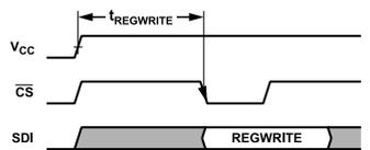
**Figure 5. Power-Up Time to Register Read Write Access**
