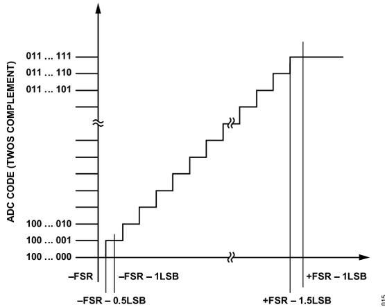
**Figure 31. ADC Ideal Transfer Function (FSR = Full-Scale Range)**
