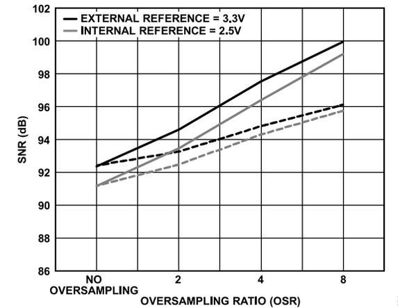
Figure 24. AD4680 SNR vs. Oversampling Ratio, Oversampling Mode
