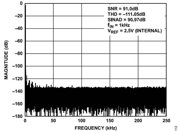
Figure 10. AD4681 FFT,  $V_{REF} = 2.5\text{ V}$  Internal
