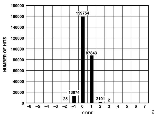
Figure 12. DC Histogram Codes at Code Center
