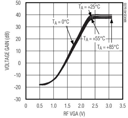
**UHF VOLTAGE GAIN vs. RF VGA VOLTAGE**
