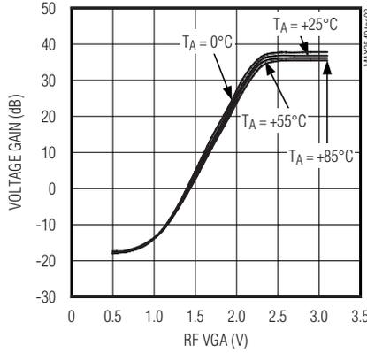
**VHF-H VOLTAGE GAIN vs. RF VGA VOLTAGE**
