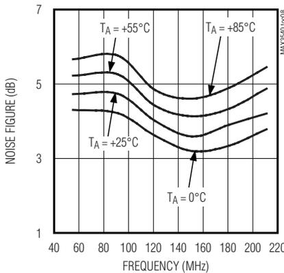
**VHF-H NOISE FIGURE vs. FREQUENCY**
