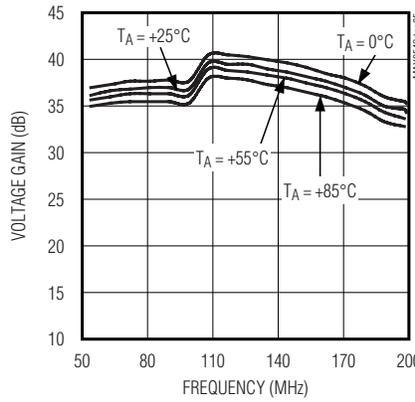
**VHF-H VOLTAGE GAIN vs. FREQUENCY**
