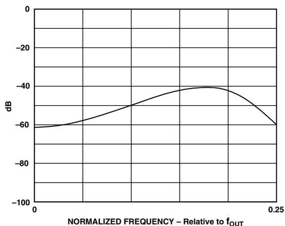
Figure 13d. Passband Frequency Response of the Decimator
