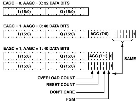
Figure 3. SSI Frame Structure
