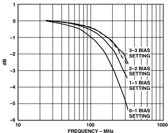
Figure 7e. LNA/Mixer Frequency Response vs. Bias Setting
