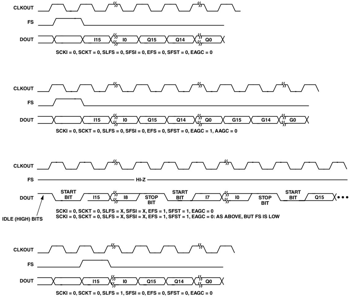
Figure 2. SSI Timing for Several SSICR Settings
