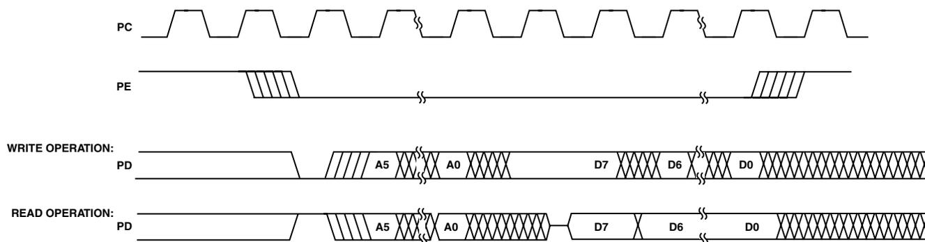
Figure 1. SPI Timing
