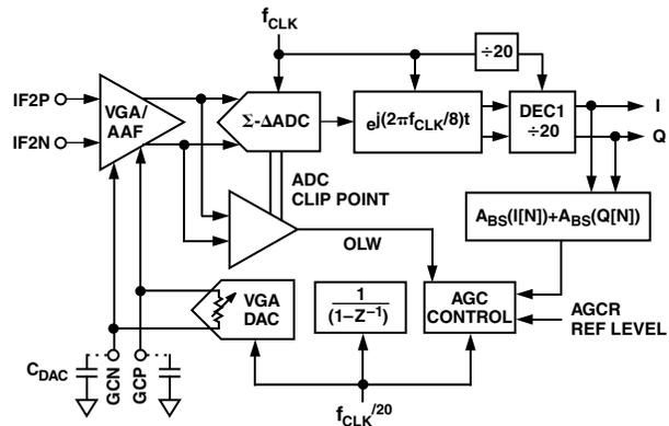
Figure 10. Functional Block Diagram of VGA and AGC
