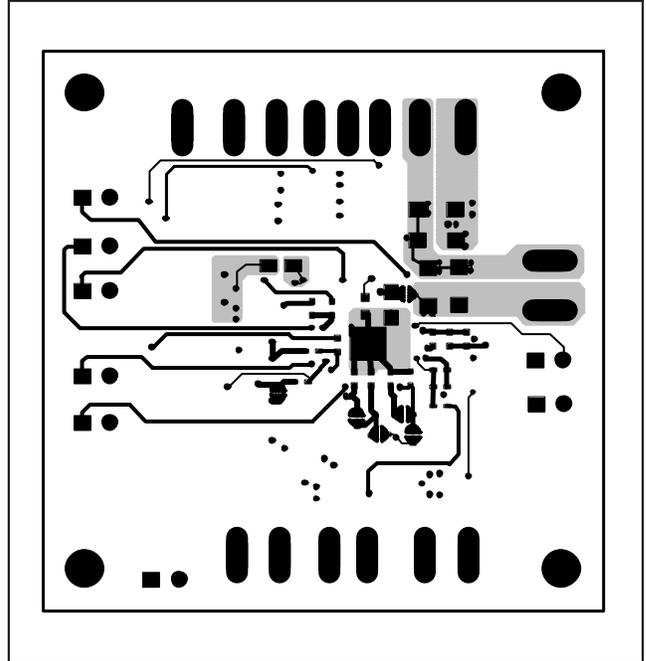
Figure 7. MAX8857A EV Kit PCB Layout—Bottom Layer
