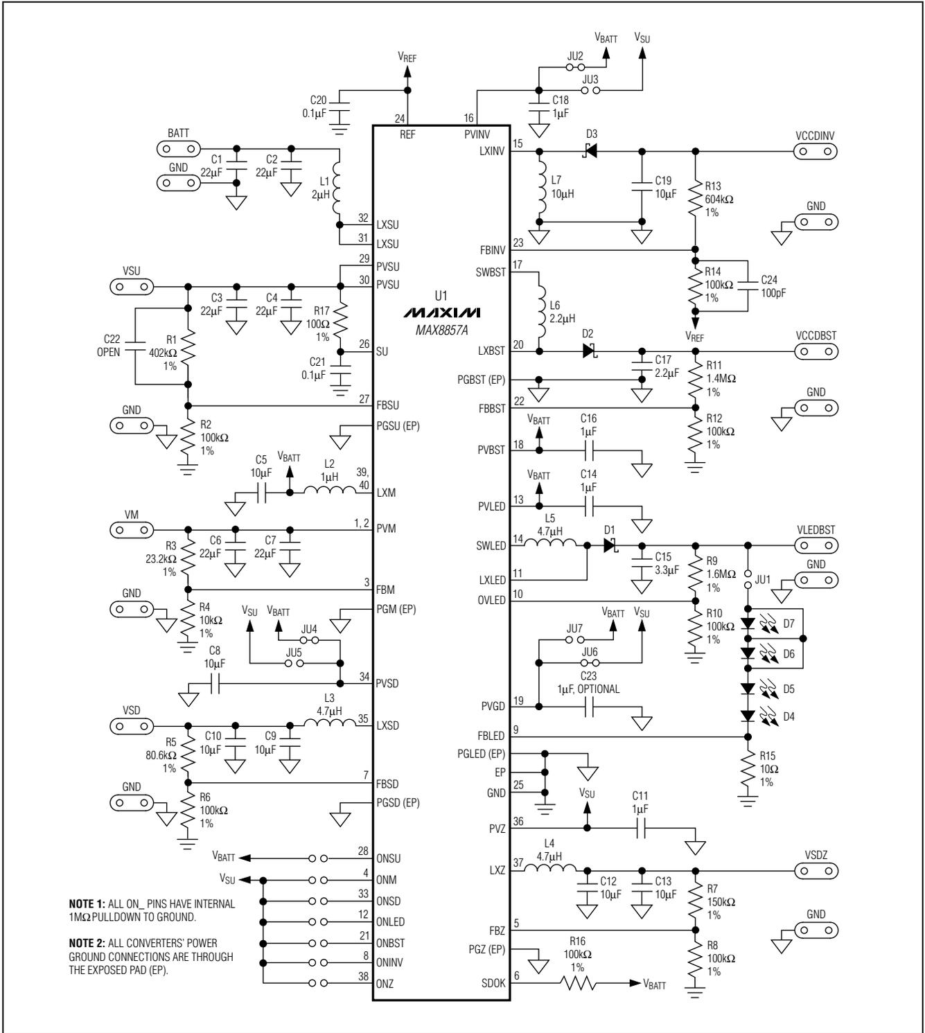
Figure 1. MAX8857A EV Kit Schematic
