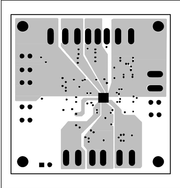
Figure 6. MAX8857A EV Kit PCB Layout—PGND Layer 3
