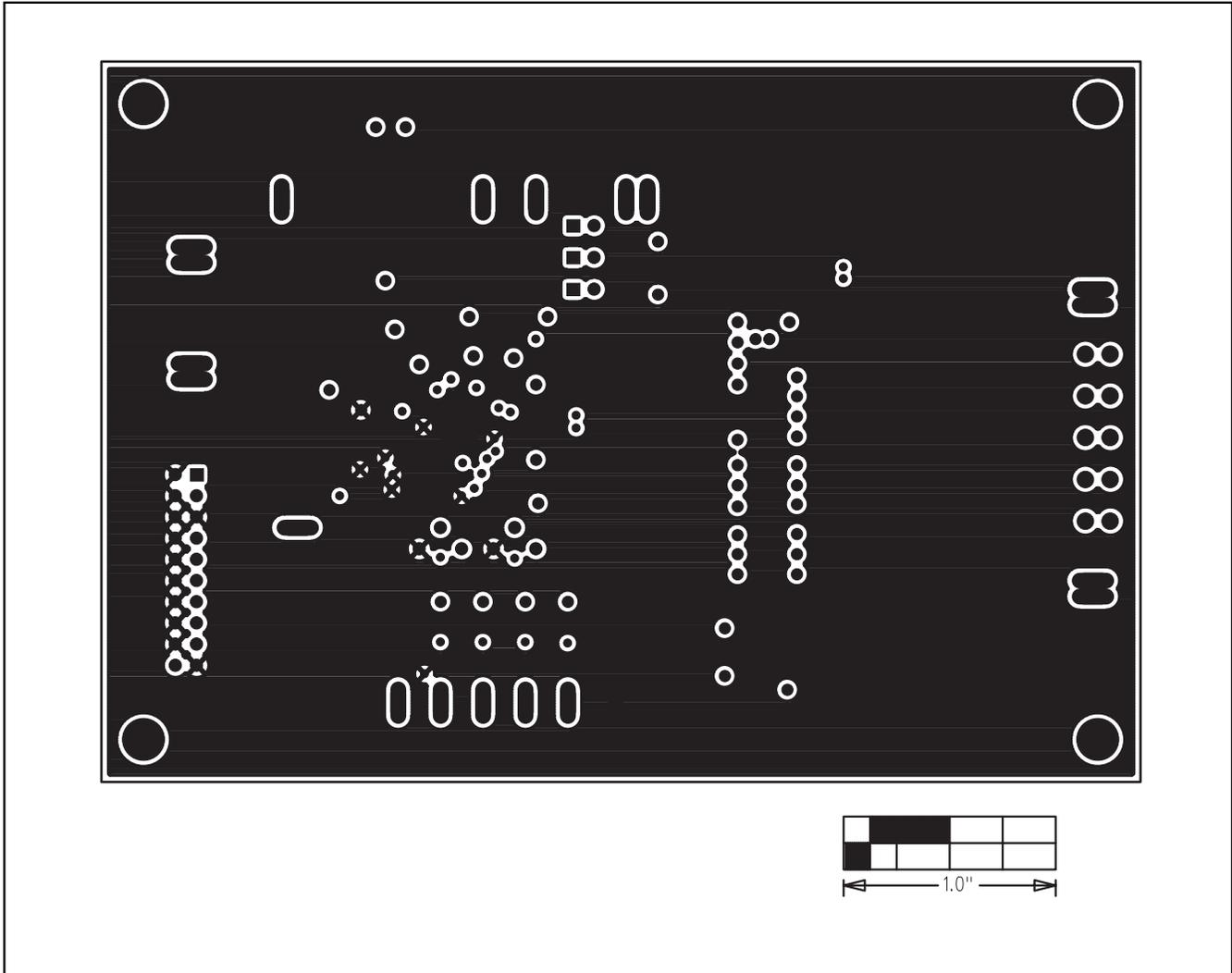
Figure 9. MAX1535D EV Kit PC Board Layout—Ground Plane
