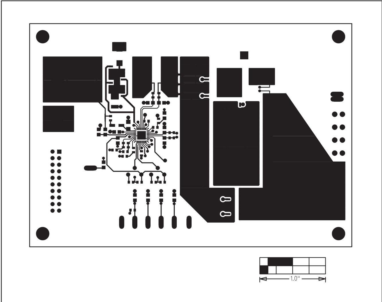
Figure 7. MAX1535D EV Kit PC Board Layout—Component Side
