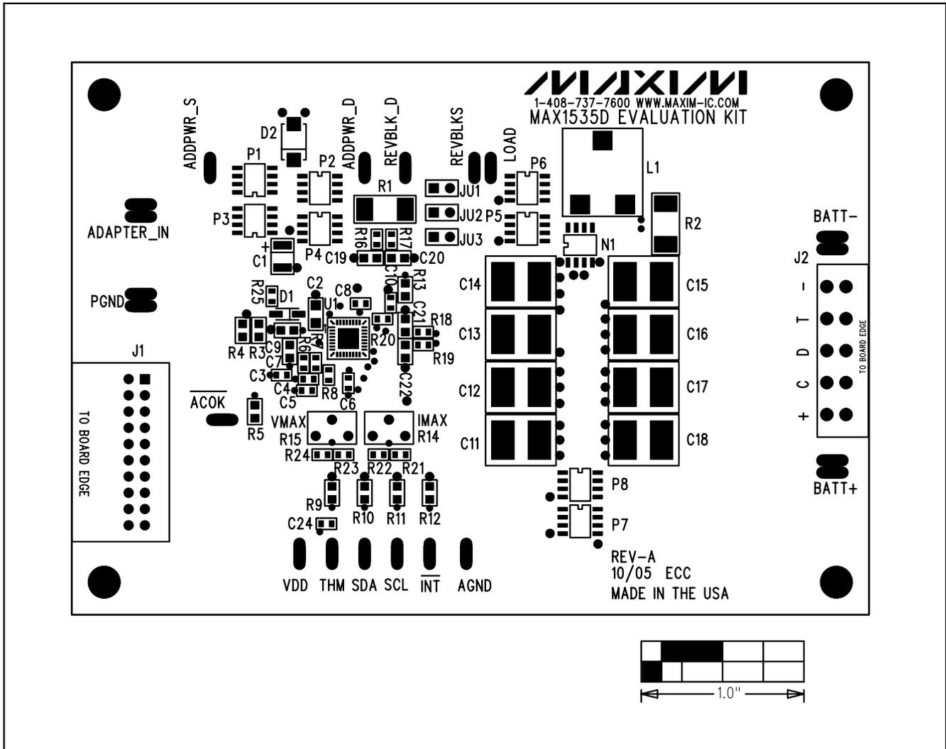
Figure 6. MAX1535D EV Kit Component Placement Guide—Component Side
