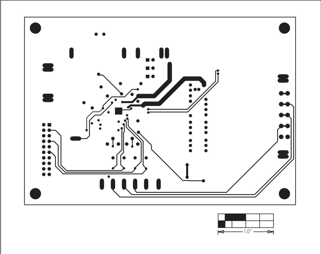
Figure 10. MAX1535D EV Kit PC Board Layout—Solder Side
