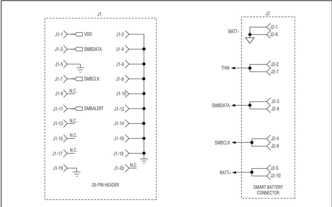
Figure 5. MAX1535D EV Kit Schematic—Smart Battery Connector
