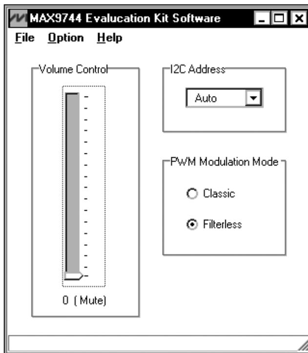
Figure 1. MAX9744 EV Kit Software GUI Window
