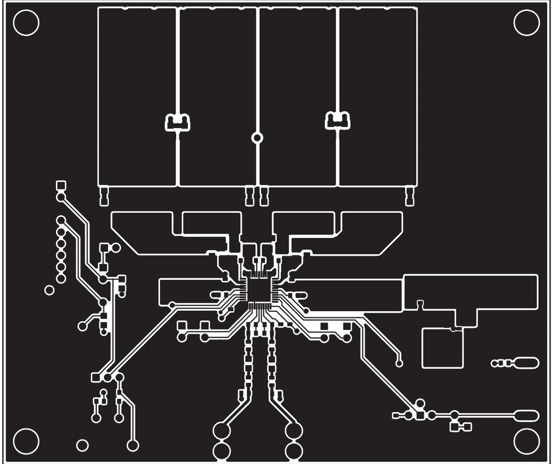
Figure 4. MAX9744 EV Kit PCB Layout—Component Side
