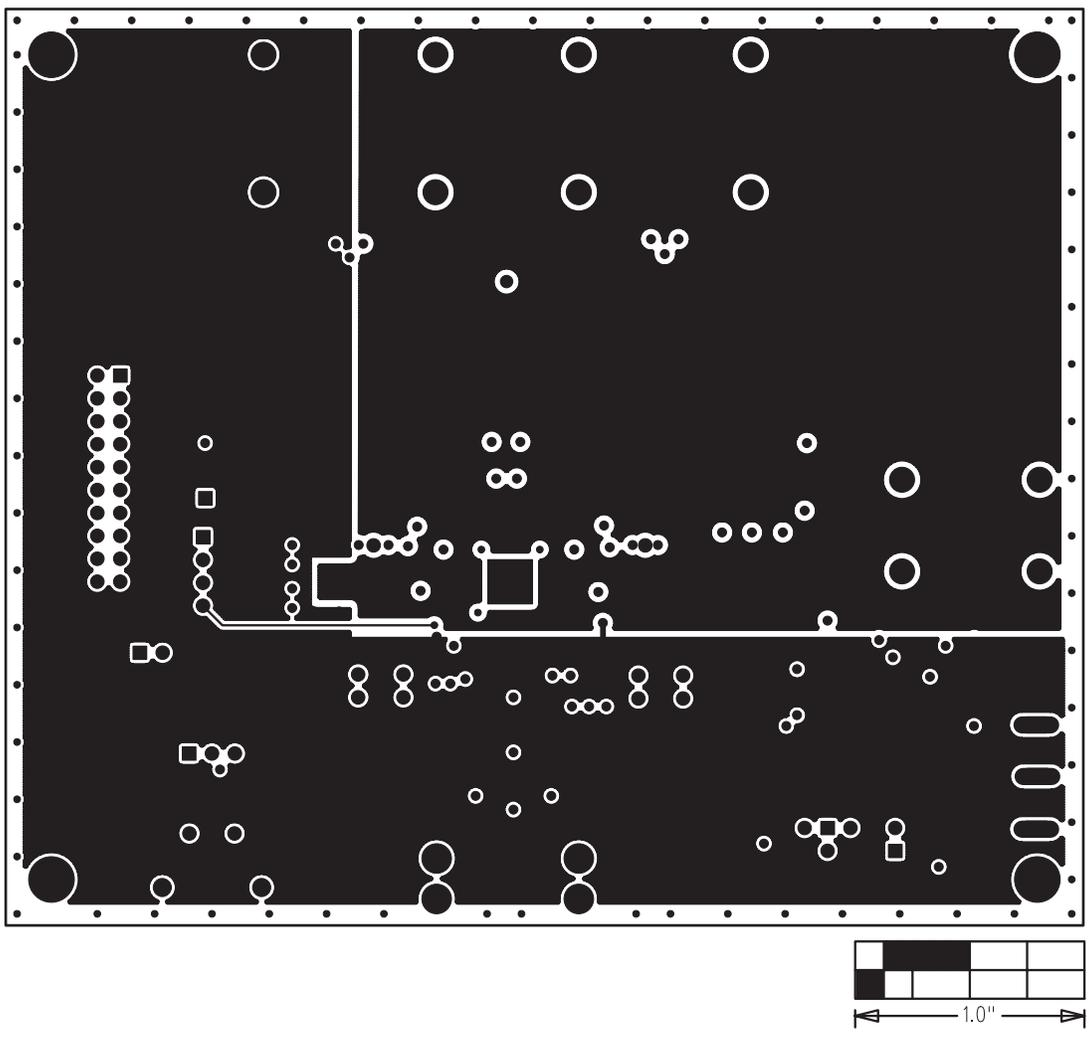
Figure 6. MAX9744 EV Kit PCB Layout—Layer 3 (Power)
