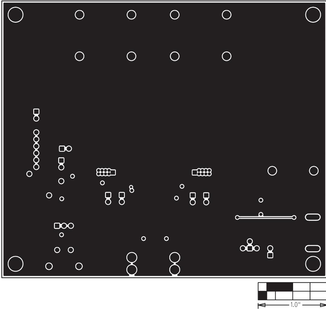
Figure 7. MAX9744 EV Kit PCB Layout—Solder Side
