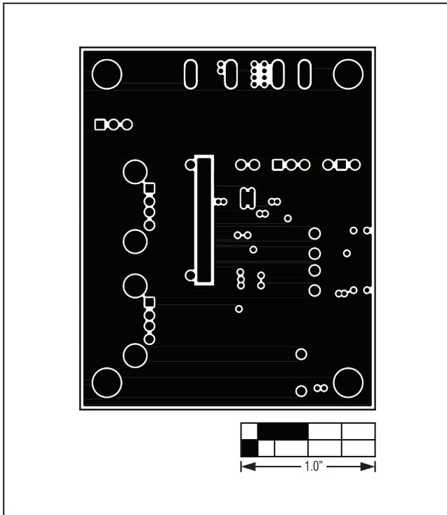
Figure 5. MAX14585 EV Kit PCB Layout—Inner Layer 3
