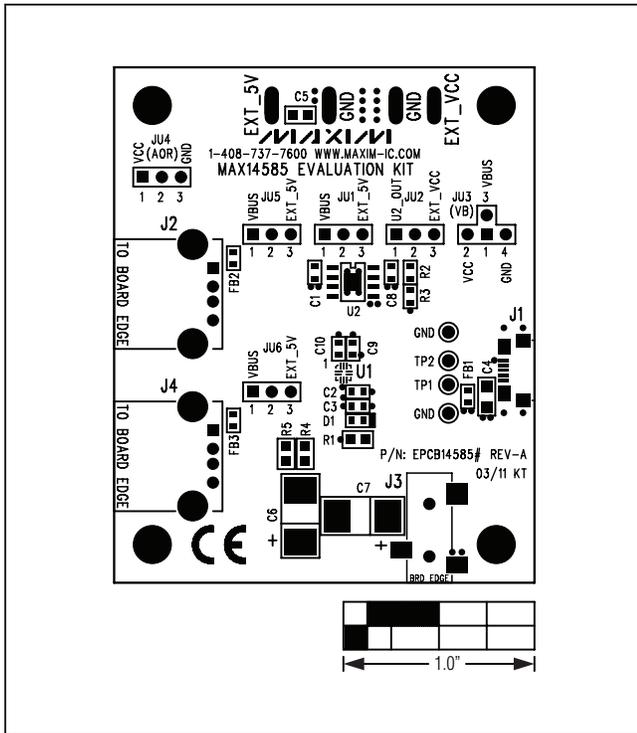
Figure 2. MAX14585 EV Kit Component Placement Guide—Component Side
