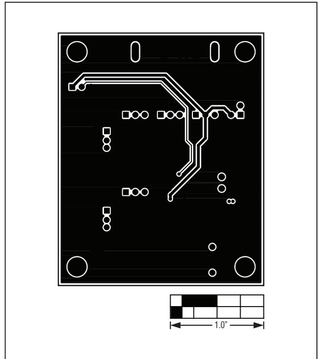
Figure 6. MAX14585 EV Kit PCB Layout—Solder Side
