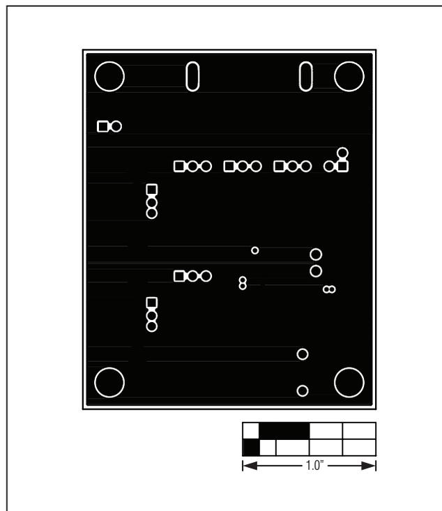
Figure 4. MAX14585 EV Kit PCB Layout—Inner Layer 2
