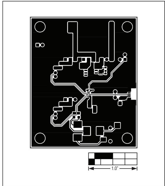
Figure 3. MAX14585 EV Kit PCB Layout—Component Side
