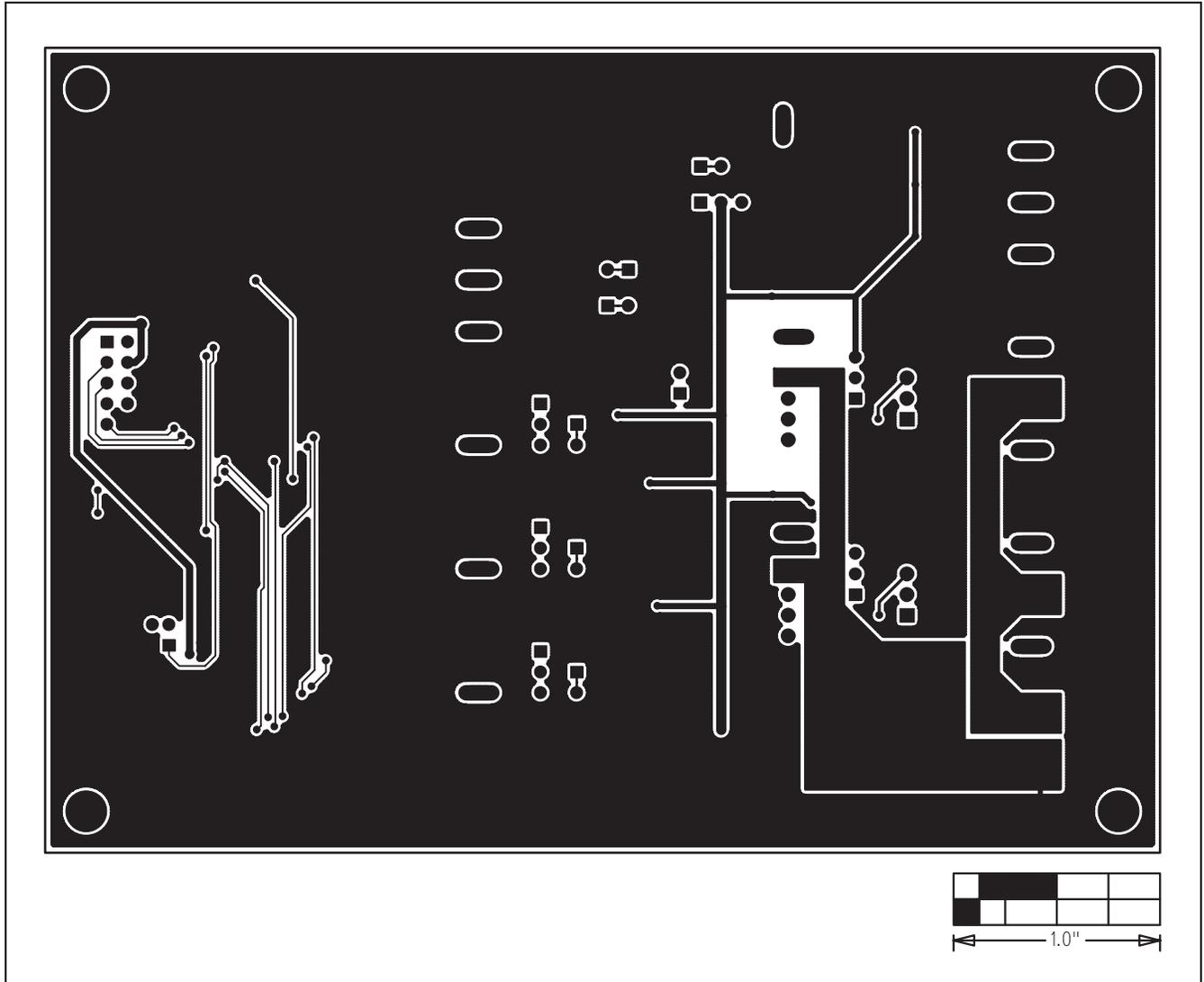
Figure 11. MAX6639 EV Kit PCB Layout—Solder Side
