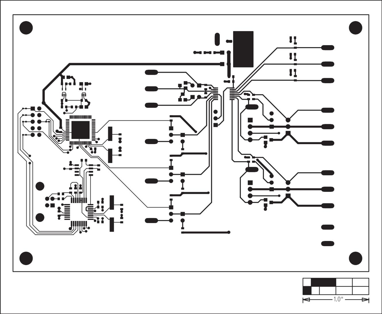
Figure 10. MAX6639 EV Kit PCB Layout—Component Side
