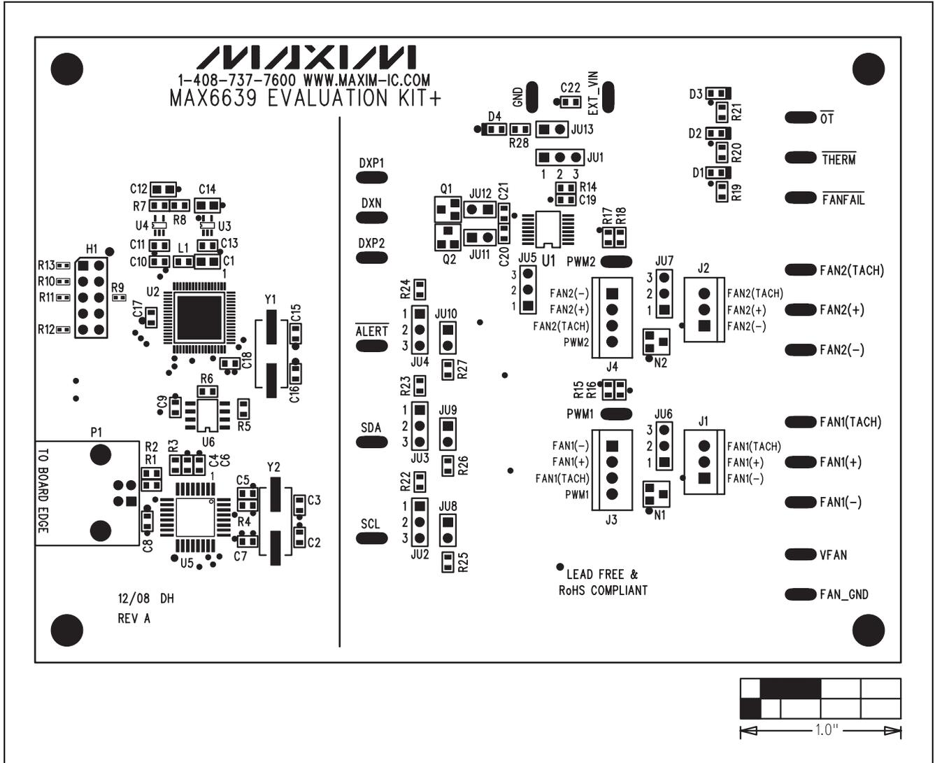
Figure 9. MAX6639 EV Kit Component Placement Guide—Component Side
