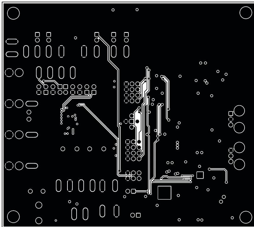
Figure 12. MAX9888 EV Kit PCB Layout—Solder Side
