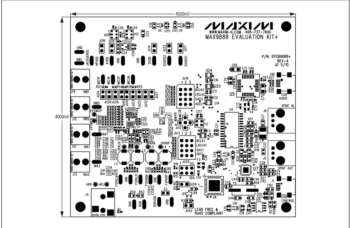
Figure 6. MAX9888 EV Kit Component Placement Guide—Component Side
