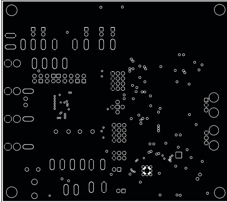
Figure 11. MAX9888 EV Kit PCB Layout—Power Layer 5
