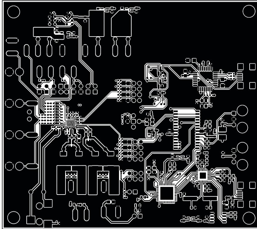
Figure 7. MAX9888 EV Kit PCB Layout—Component Side
