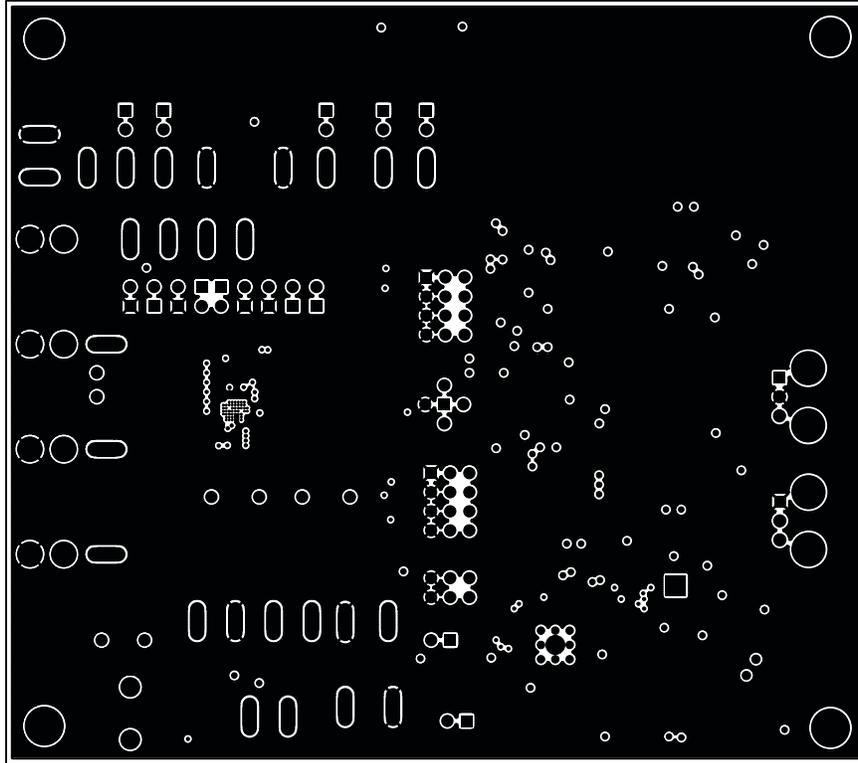
Figure 8. MAX9888 EV Kit PCB Layout—Ground Layer 2
