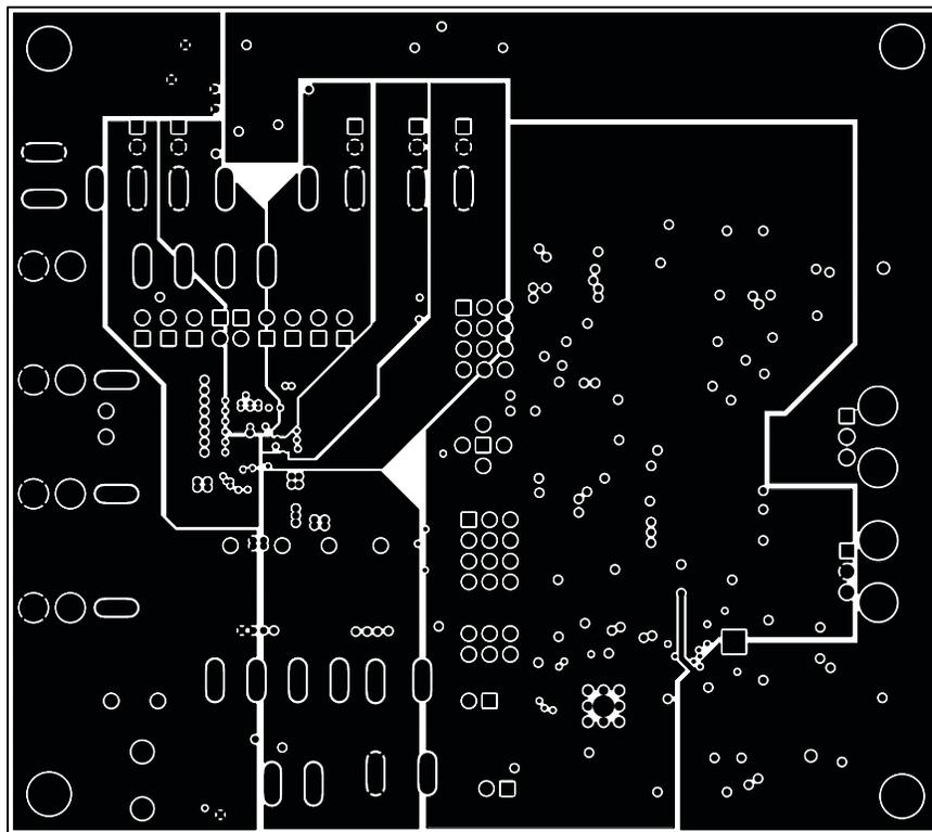
Figure 10. MAX9888 EV Kit PCB Layout—Power Layer 4
