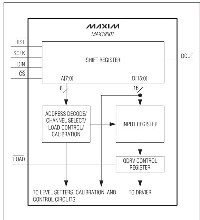
Figure 2. Serial-Interface Block Diagram
