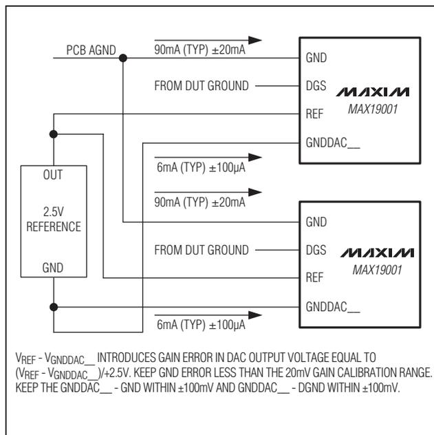
Figure 7. Sample Connection Diagram for Two Parts per Board
