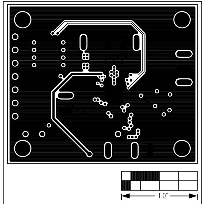
Figure 5. MAX17019N EV Kit PCB Layout—Layer 3
