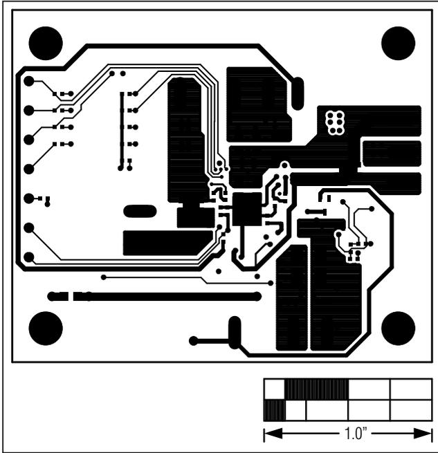
Figure 6. MAX17019N EV Kit PCB Layout—Solder Side
