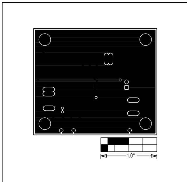
Figure 5. MAX15040 EV Kit PCB Layout—Inner Layer 3
