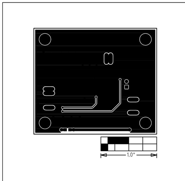
Figure 6. MAX15040 EV Kit PCB Layout—Solder Side
