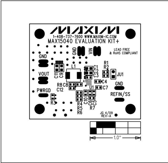
Figure 2. MAX15040 EV Kit Component Placement Guide—Component Side
