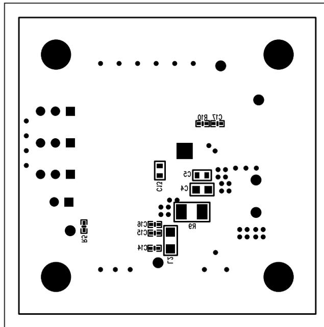
Figure 7. MAX20003 EV Kit Component Placement Guide—Solder Side
