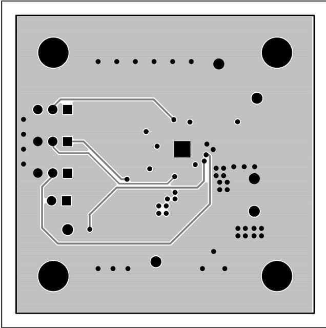
Figure 5. MAX20003 EV Kit PCB Layout—Layer 3
