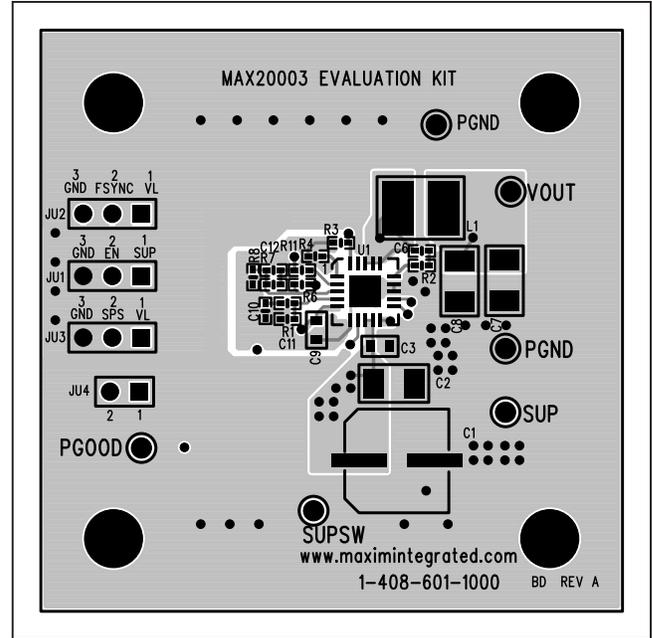
Figure 3. MAX20003 EV Kit PCB Layout—Component Side
