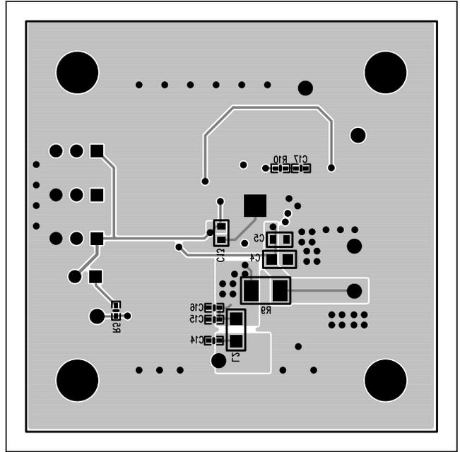
Figure 6. MAX20003 EV Kit PCB Layout—Solder Side
