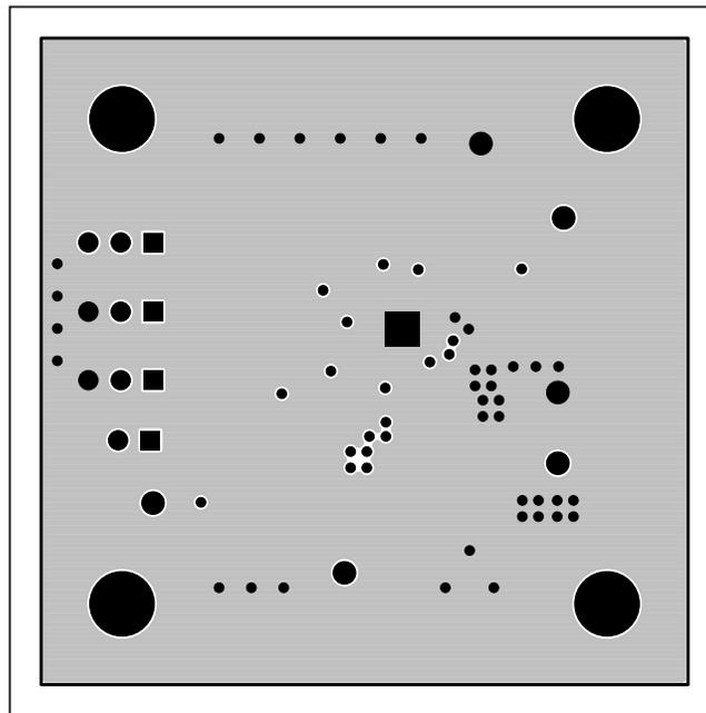
Figure 4. MAX20003 EV Kit PCB Layout—Layer 2
