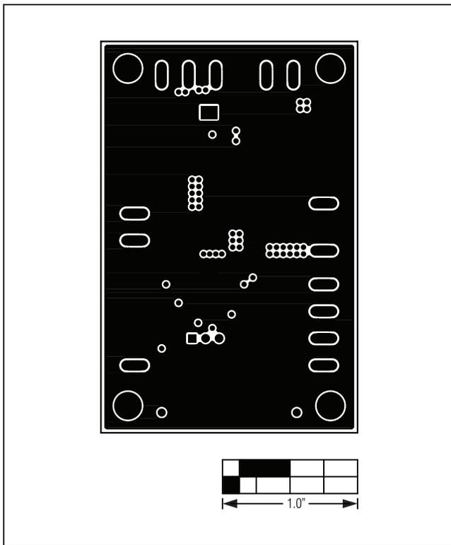
Figure 4. MAX17512 EV Kit PCB Layout—Layer 2
