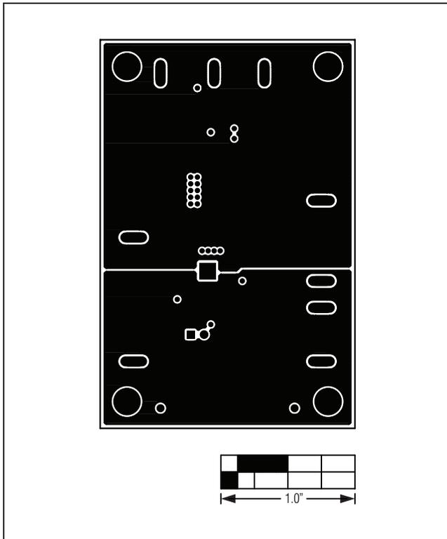
Figure 6. MAX17512 EV Kit PCB Layout—Layer 4
