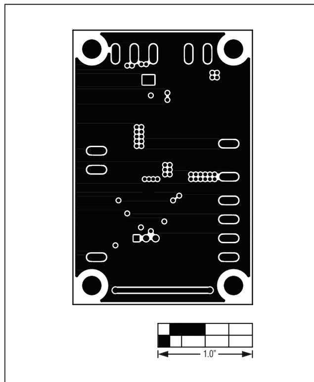
Figure 8. MAX17512 EV Kit PCB Layout—Solder Side
