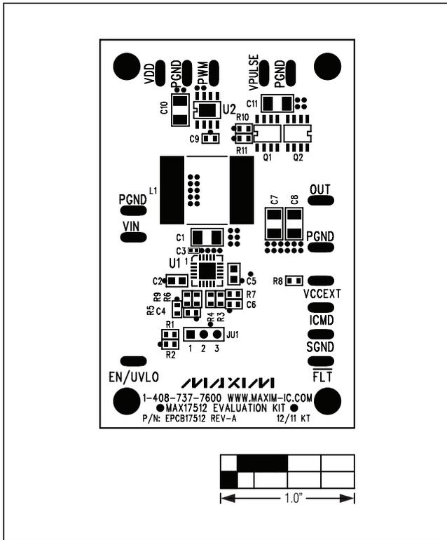
Figure 2. MAX17512 EV Kit Component Placement Guide—Component Side
