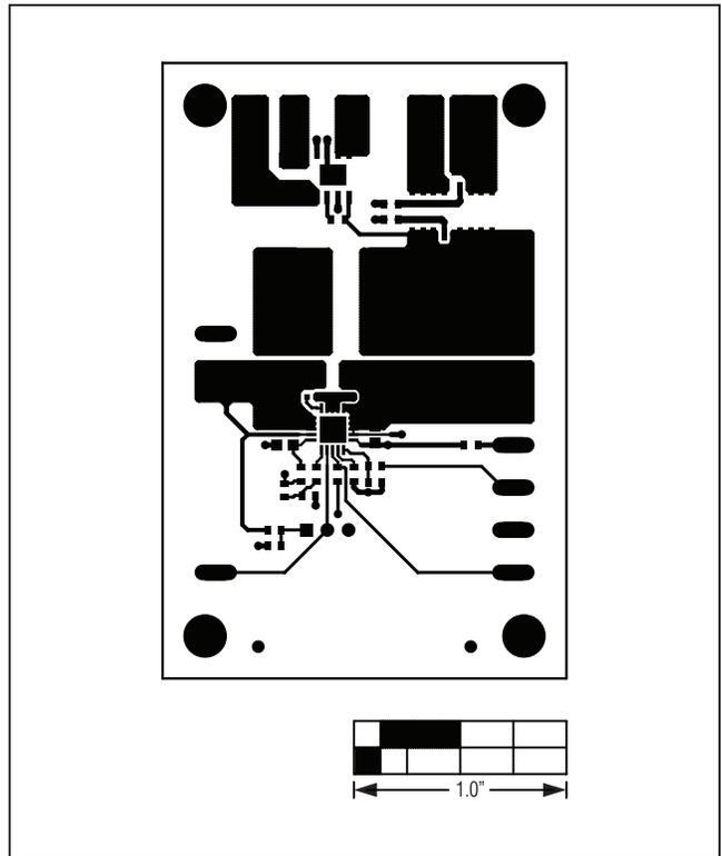
Figure 3. MAX17512 EV Kit PCB Layout—Component Side
