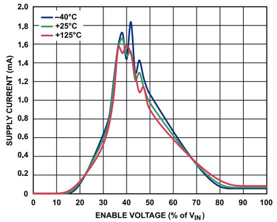
Figure 31. Supply Current vs. ENABLE Pin Voltage
