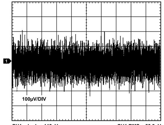
Figure 19. ADR3550 Output Voltage Noise (10 Hz to 10 kHz)
