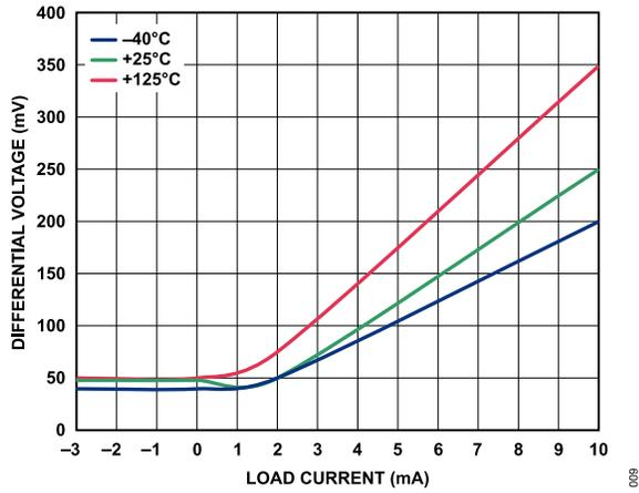
Figure 9. ADR3525 Dropout Voltage vs. Load Current
