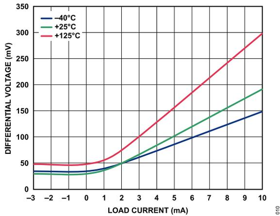
Figure 10. ADR3550 Dropout Voltage vs. Load Current
