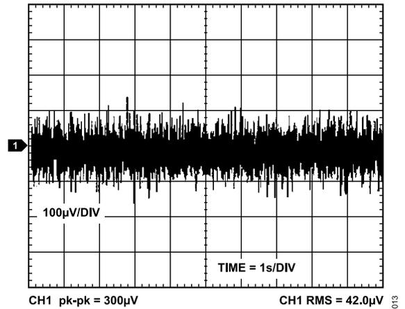
Figure 13. ADR3525 Output Voltage Noise (10 Hz to 10 kHz)
