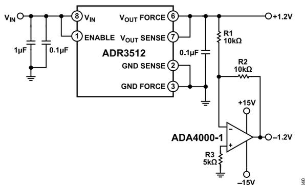
Figure 40. Bipolar Output Reference
