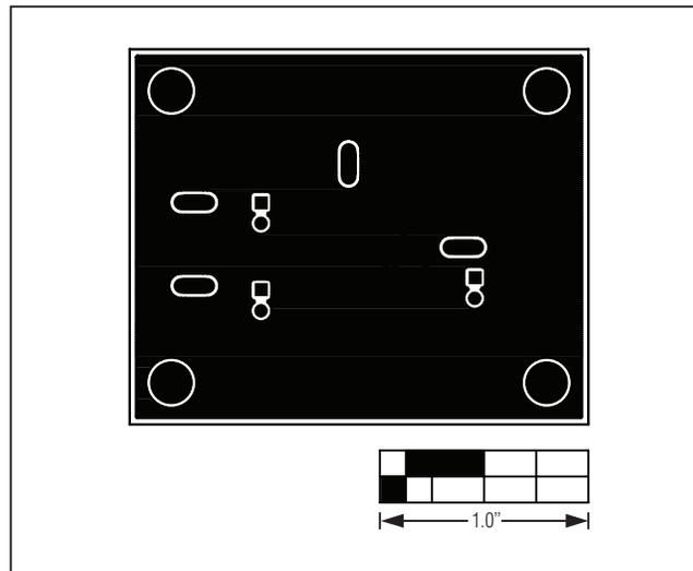
Figure 4. MAX16910C9 EV Kit PCB Layout—Solder Side
