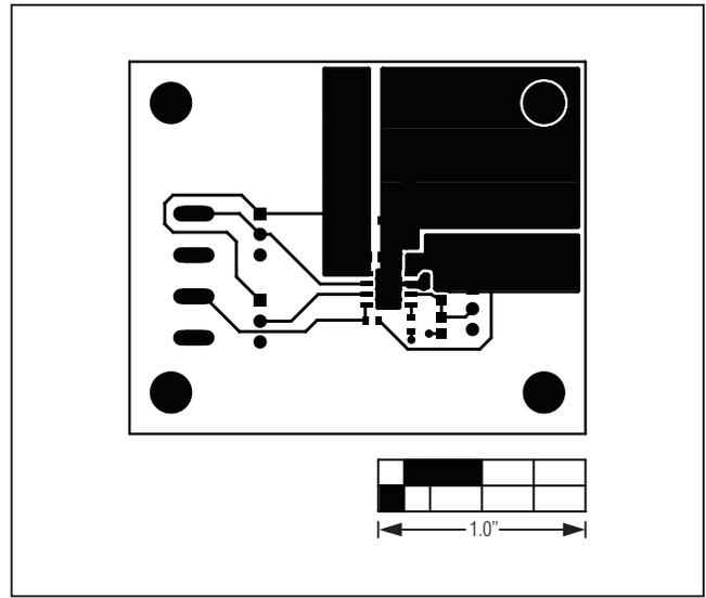
Figure 3. MAX16910C9 EV Kit PCB Layout—Component Side
