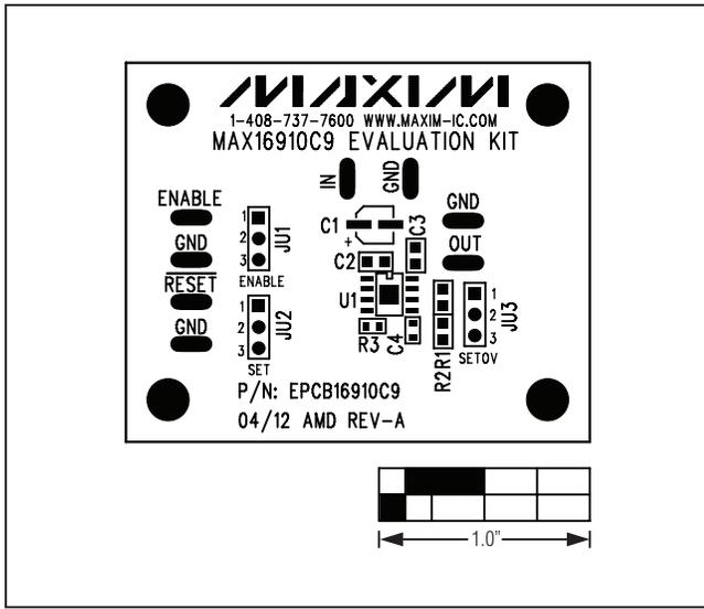
Figure 2. MAX16910C9 EV Kit Component Placement Guide—Silkscreen
