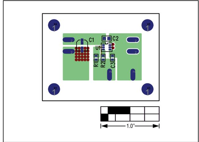
Figure 3. MAX5048C EV Kit PCB Layout—Component Side
