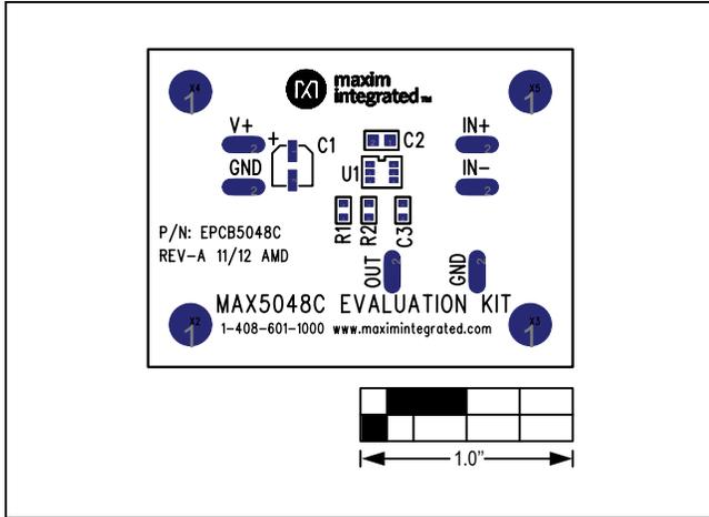
Figure 2. MAX5048C EV Kit Component Placement—Component Side
