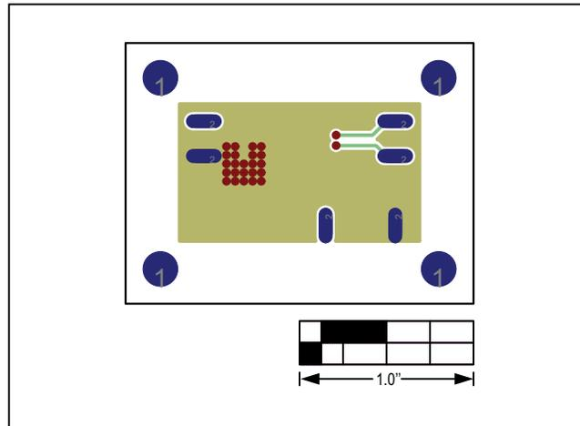
Figure 4. MAX5048C EV Kit PCB Layout—Solder Side
