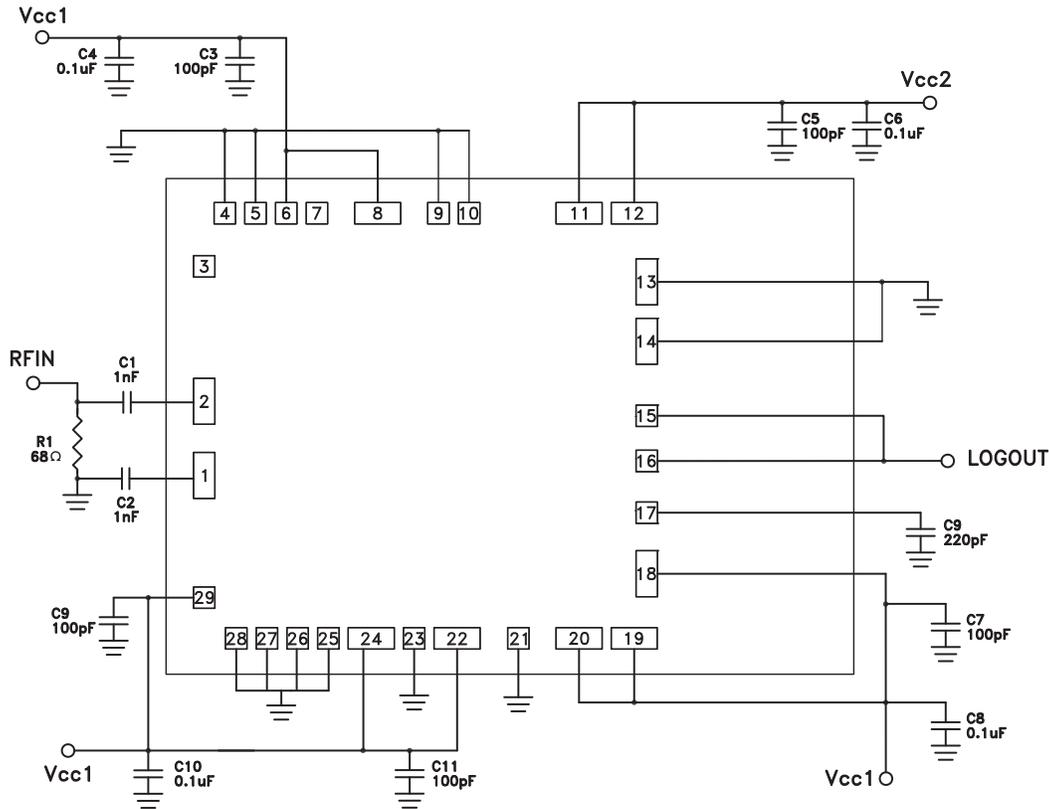
Note 1: For detector mode, connect high impedance volt meter to the LOGOUT port. LOGOUT is shorted to VSET, as required for detector mode.
