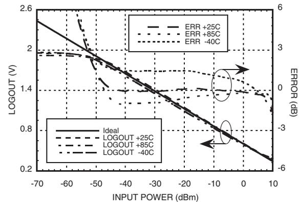
Unless otherwise noted:  $V_{cc1}, V_{cc2} = +5V, T_A = +25C$
