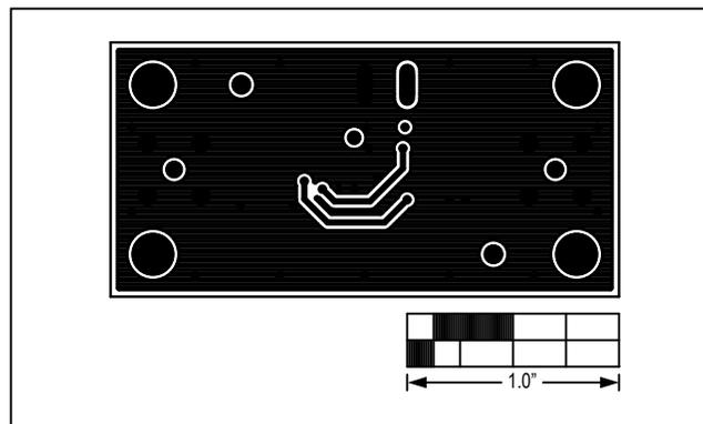
Figure 4. MAX44281V EV Kit PCB Layout—Solder Side
