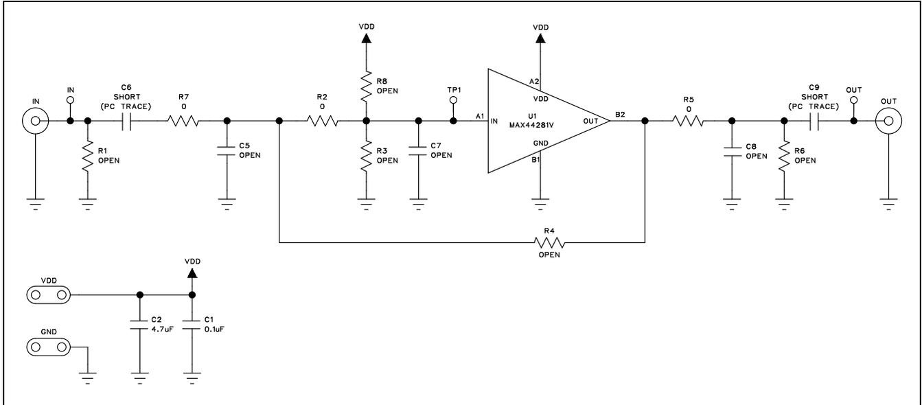
Figure 1. MAX44281V EV Kit Schematic
