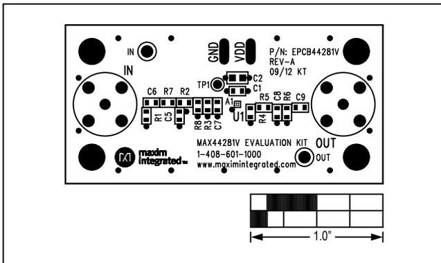
Figure 2. MAX44281V EV Kit Component Placement Guide—Component Side
