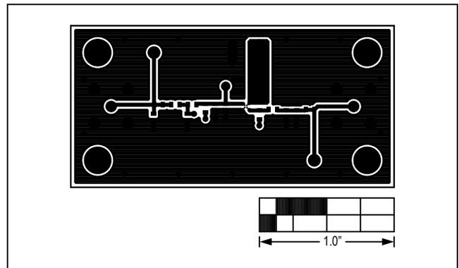
Figure 3. MAX44281V EV Kit PCB Layout—Component Side
