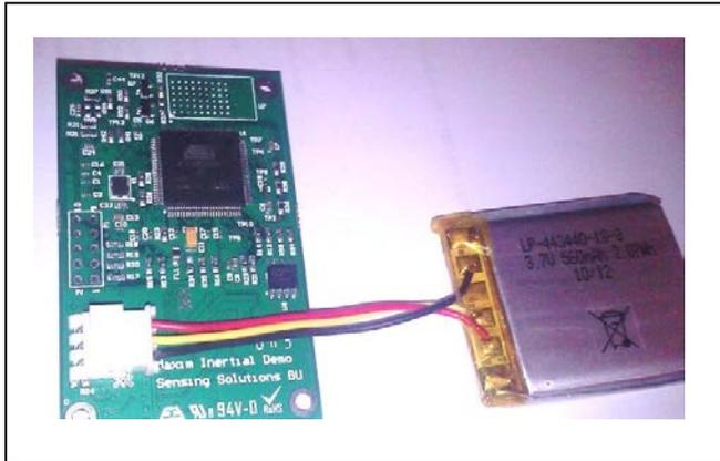
Figure 32. Battery Connection
