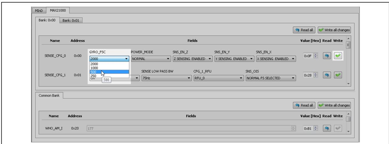
Figure 17. Sets the Gyroscope to Full Scale on the MAX21000
