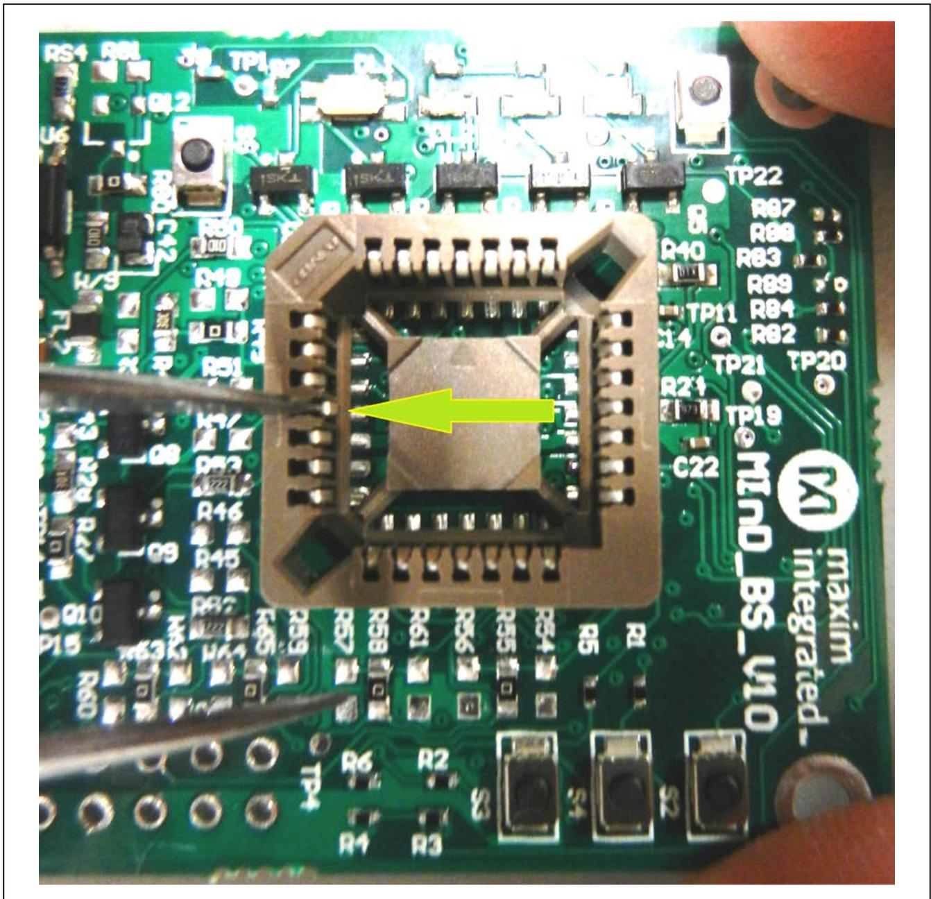
Figure 1. PLCC28 Folding for Electrical Contact Improvement
