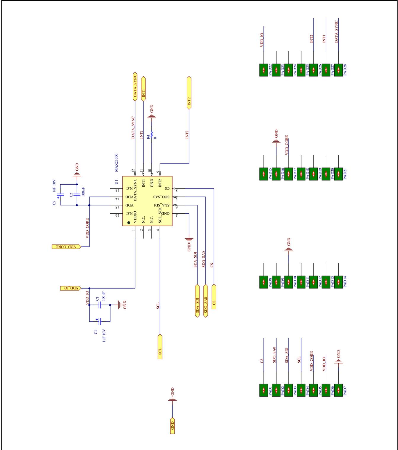
Figure 39. MAX21000 MInD EV Kit STAMP Board Support Schematic
