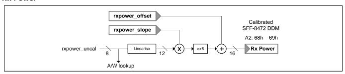
Figure 18. Calculating the Rx Power DDM
