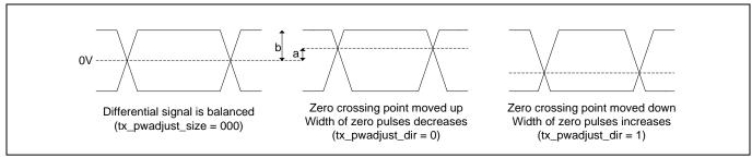
Figure 6. Crossing Point Adjustment
