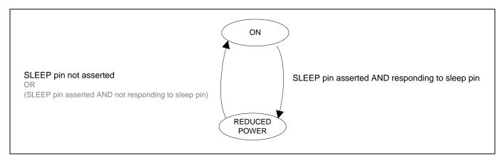
Figure 21. Conditions for Moving In and Out of Sleep Mode
