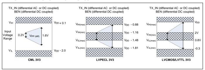
Typical I/O ranges for TX\_IN and BEN are shown. TX\_IN and BEN inputs are also compatible with HSTL and SSTL for low voltage operation.
