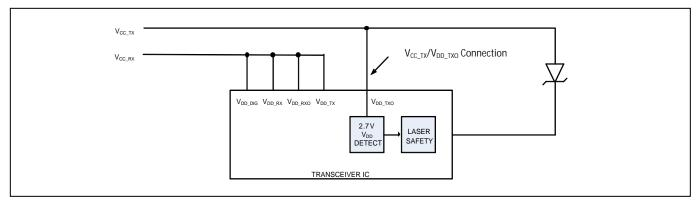
Figure 13. V<sub>DD TXO</sub> Configured to Assert Laser Shutdown
