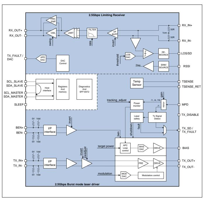
Figure 1. MAX24003 Block Diagram
