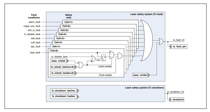
Figure 12. Laser Safety System
