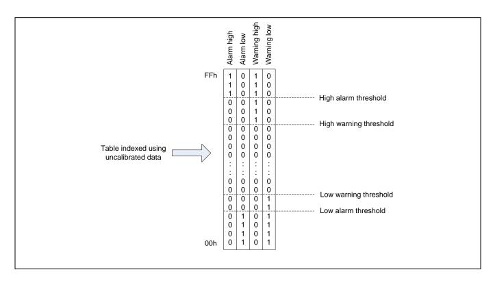
Figure 19. Using 8-Bit Calibrated Data to Look Up Alarm and Warning Flags
