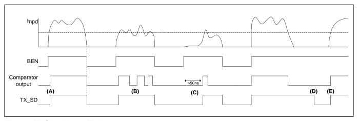
Figure 9. TX Signal Detect Timing
