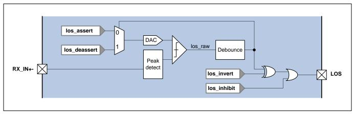
Figure 3. LOS Detection System
