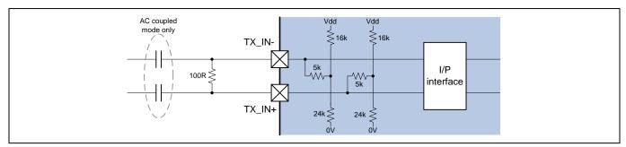
Figure 5. TX\_IN and BEN Input Termination and Signal Conditioning
