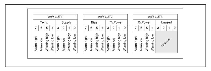
Figure 20. Alarm and Warning LUT Mapping
