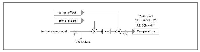
Figure 14. Calculating the Temperature DDM
