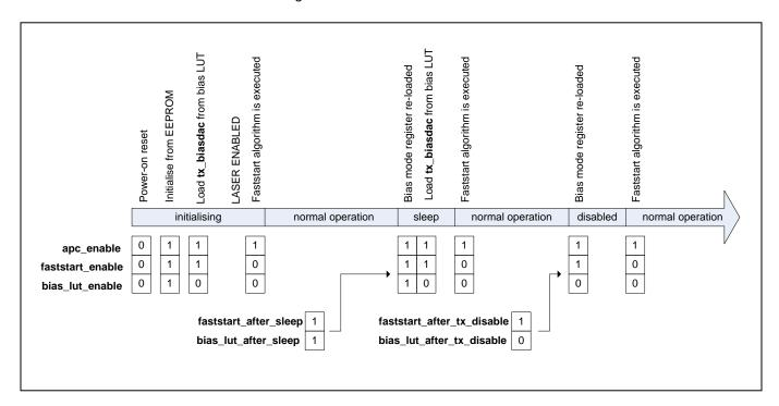
Figure 10. Behavior of the tx\_biasmode Register in Closed-Loop Mode
