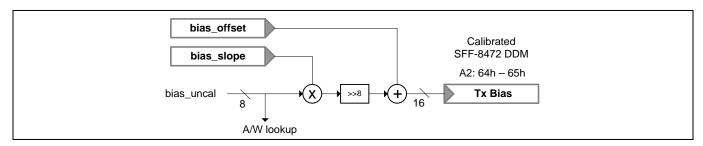
Figure 16. Calculating the Bias Current DDM
