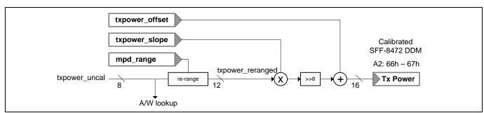
Figure 17. Calculating the Tx Power DDM
