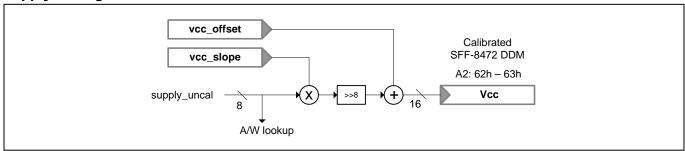
Figure 15. Calculating the Supply Voltage DDM
