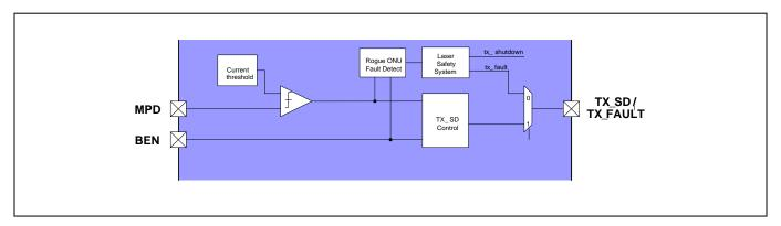
Figure 7. TX SD Pin Signal Generation
