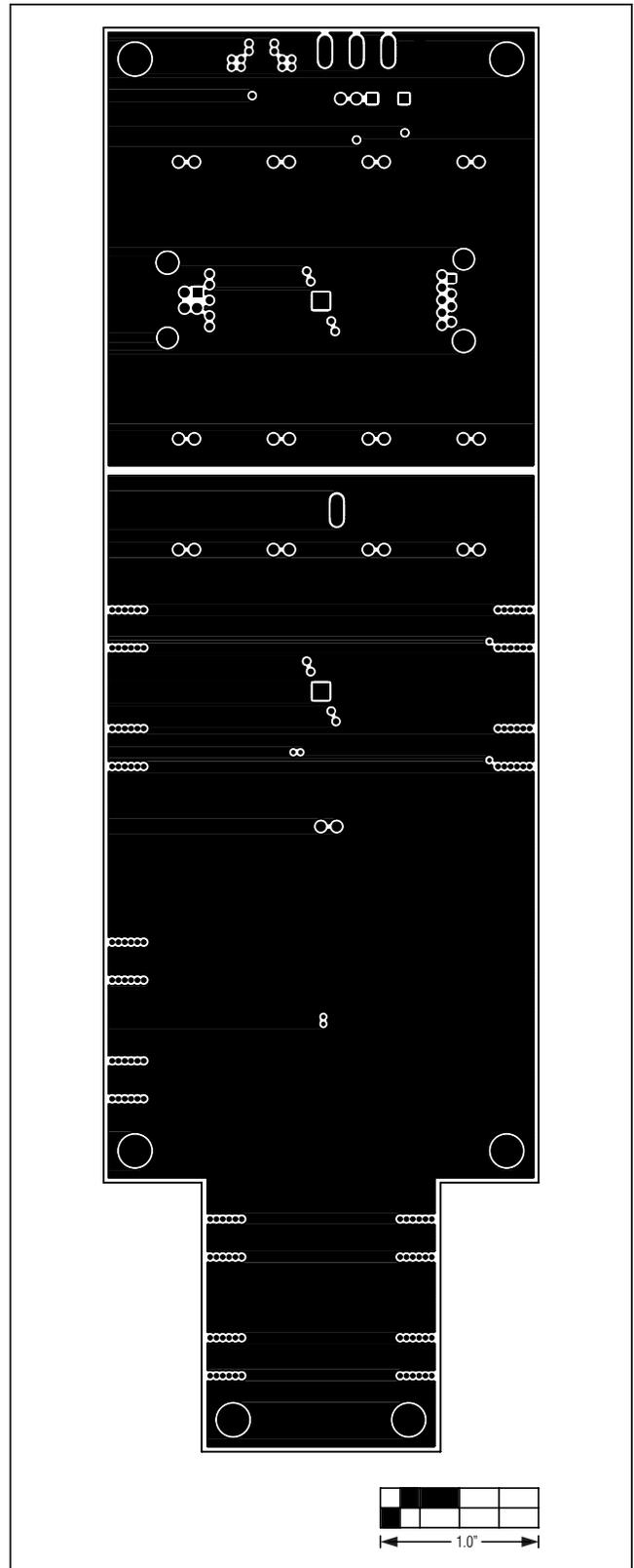
Figure 5. MAX14972 EV Kit PCB Layout—Inner Layer 3
