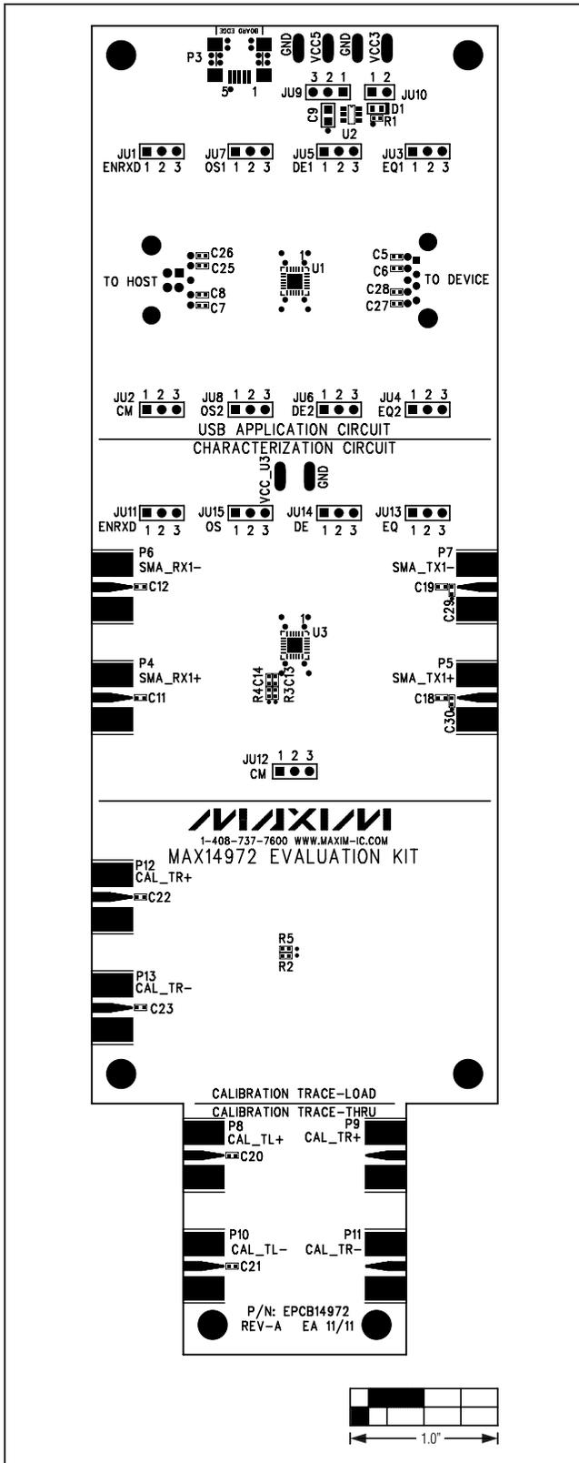
Figure 2. MAX14972 EV Kit Component Placement Guide—Component Side
