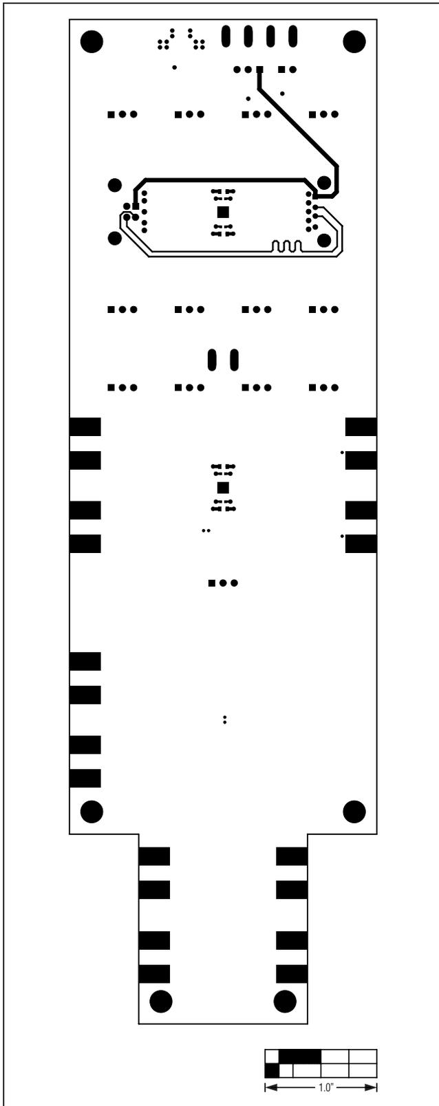
Figure 6. MAX14972 EV Kit PCB Layout—Solder Side
