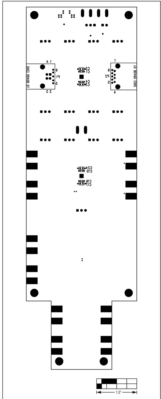
Figure 7. MAX14972 EV Kit Component Placement Guide—Solder Side
