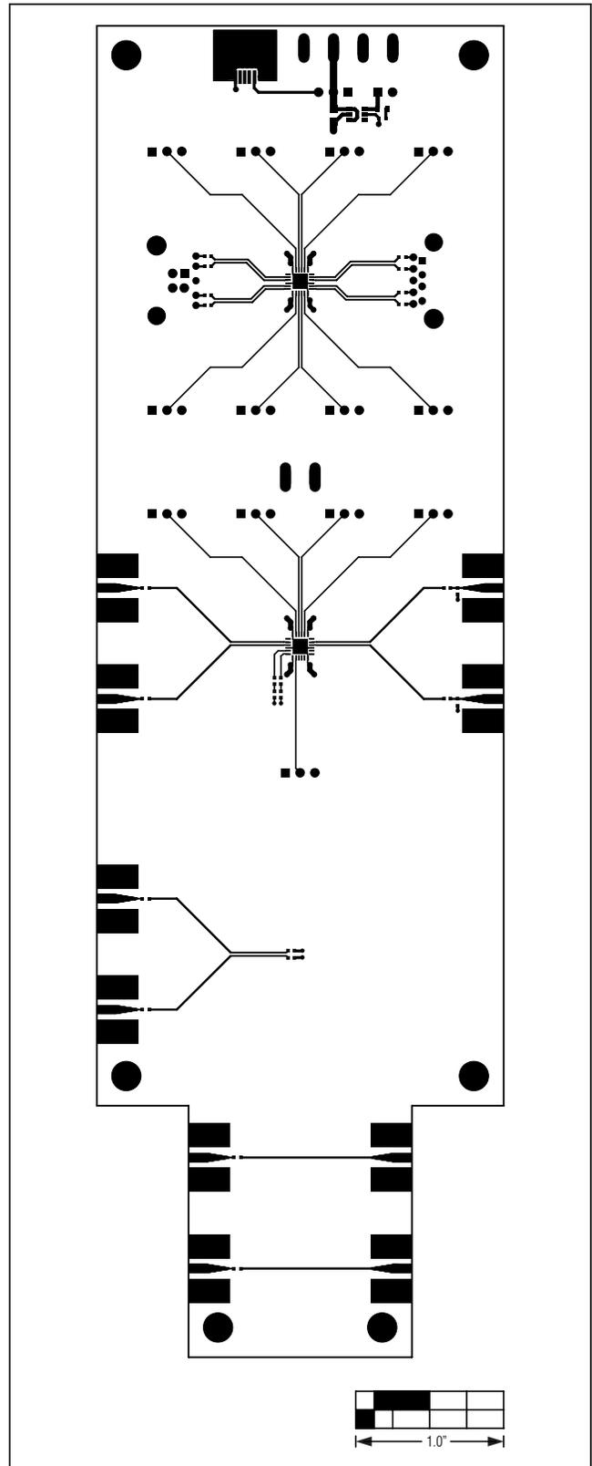
Figure 3. MAX14972 EV Kit PCB Layout—Component Side
