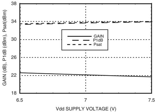
**Gain & Power vs. Supply Current @ 8 GHz**
