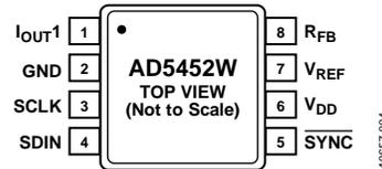
Figure 3. Pin Configuration
