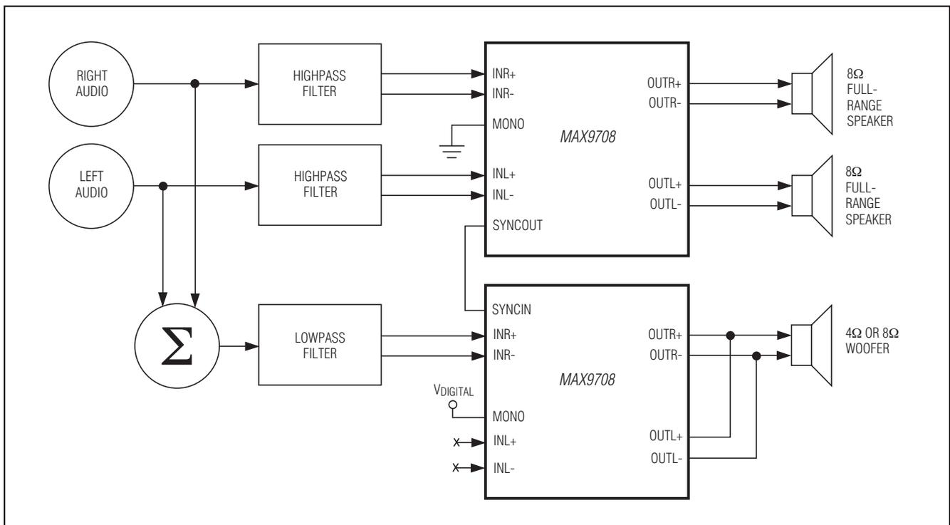
Figure 5. Multiple Amplifiers Implement a 2.1 Audio System
