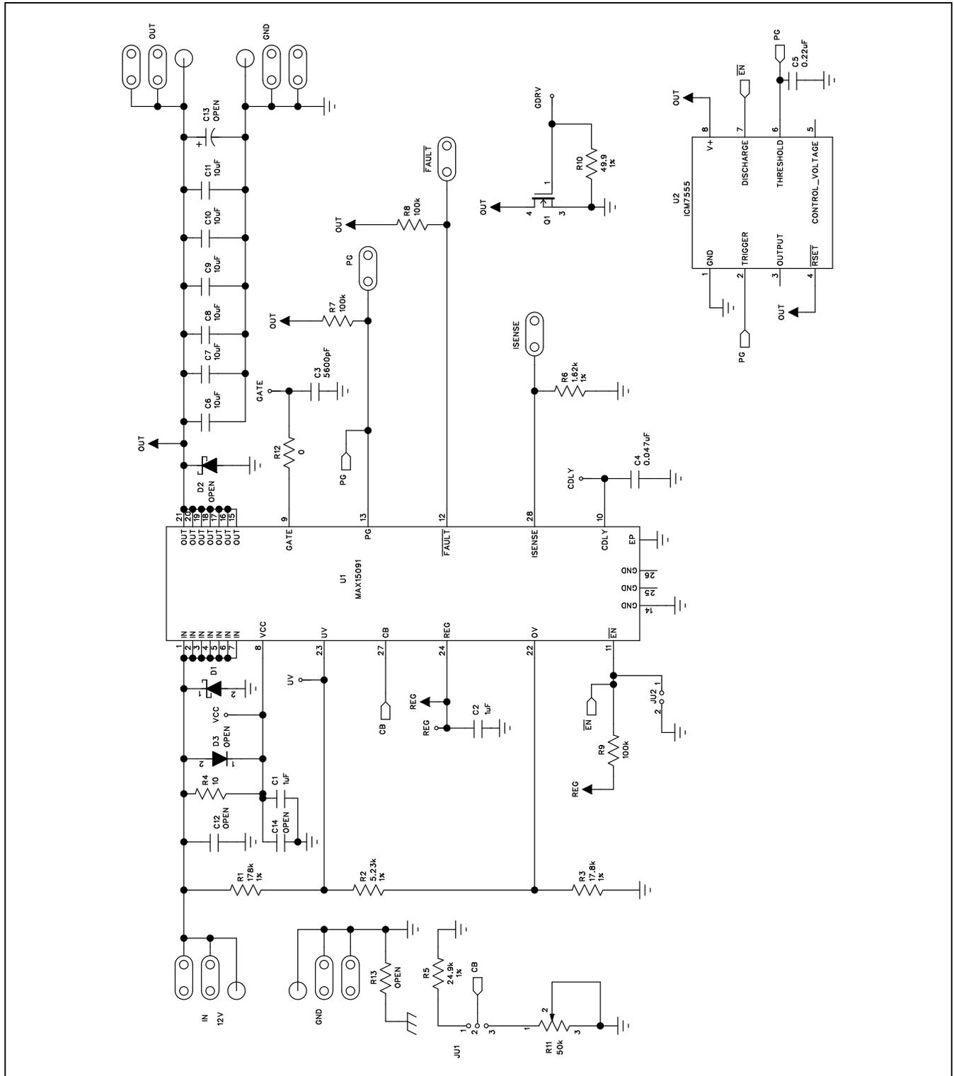
Figure 1. MAX15091 EV Kit Schematic
