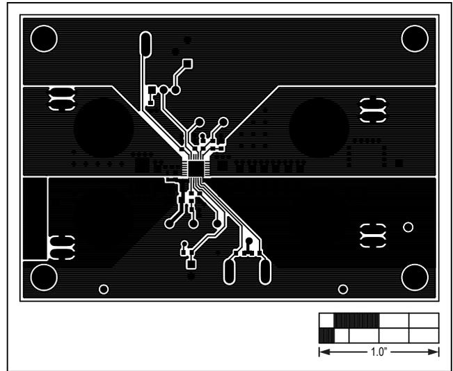
Figure 3. MAX15091 EV Kit PCB Layout—Component Side
