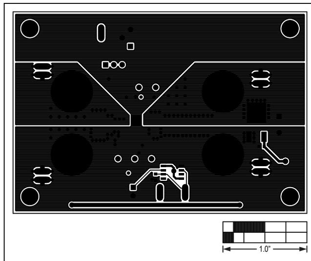
Figure 6. MAX15091 EV Kit PCB Layout—Solder Side
