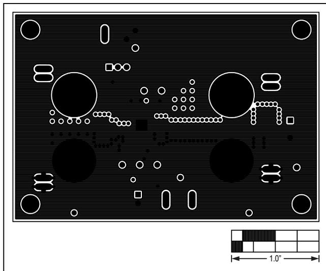
Figure 5. MAX15091 EV Kit PCB Layout—Layer 3 (GND)
