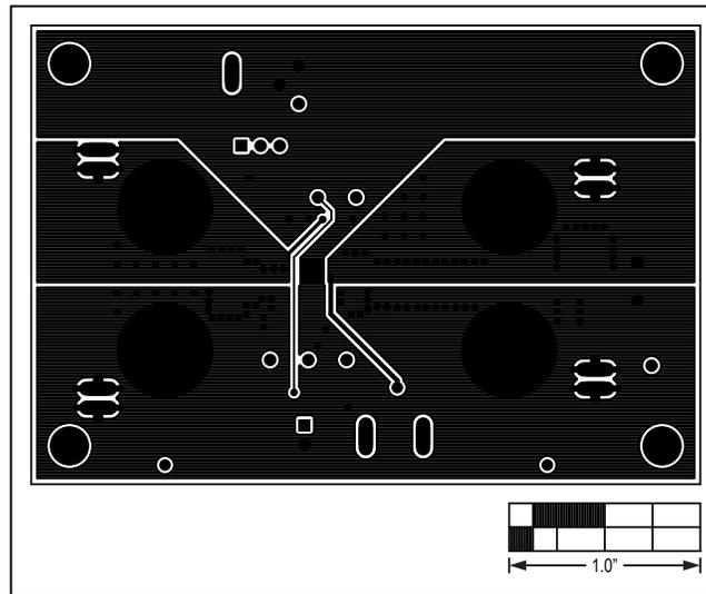
Figure 4. MAX15091 EV Kit PCB Layout—Layer 2 (PWR/GND)
