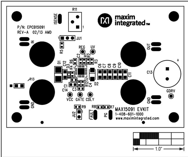
Figure 2. MAX15091 EV Kit Component Placement Guide—Component Side
