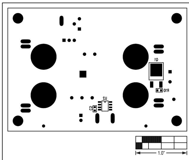
Figure 7. MAX15091 EV Kit Component Placement Guide—Solder Side
