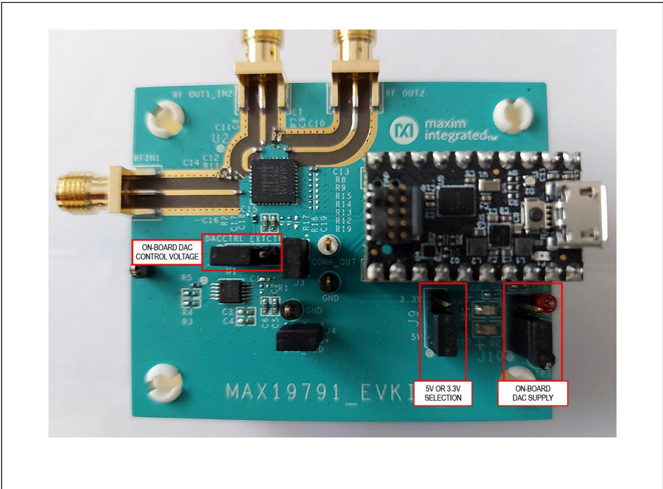
Figure 4. Connection Setup for Using On-Board Power Supply and On-Board Control Voltage
