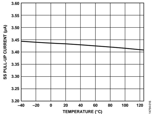
Figure 16. SS Pin Pull-Up Current vs. Temperature
