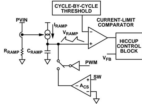
Figure 35. Current-Limit Circuit
