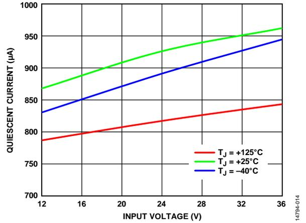
Figure 14. Quiescent Current vs. Input Voltage ( $V_{PVIN}$ )
