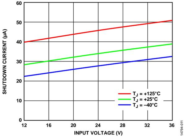
Figure 11. Shutdown Current vs. Input Voltage ( $V_{PVIN}$ )
