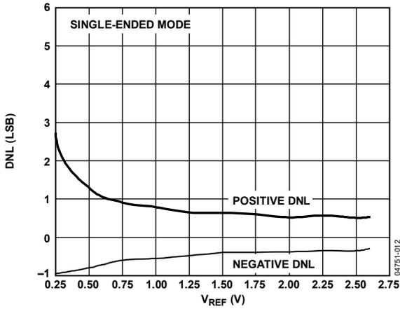
Figure 10. AD7938-6 DNL vs.  $V_{REF}$  for  $V_{DD} = 3V$
