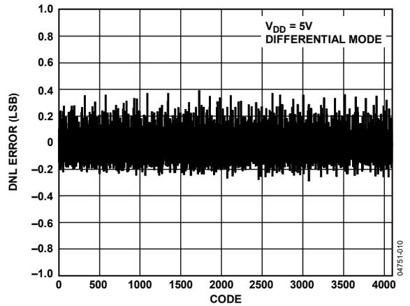
Figure 8. AD7938-6 Typical DNL at V<sub>DD</sub> = 5 V
