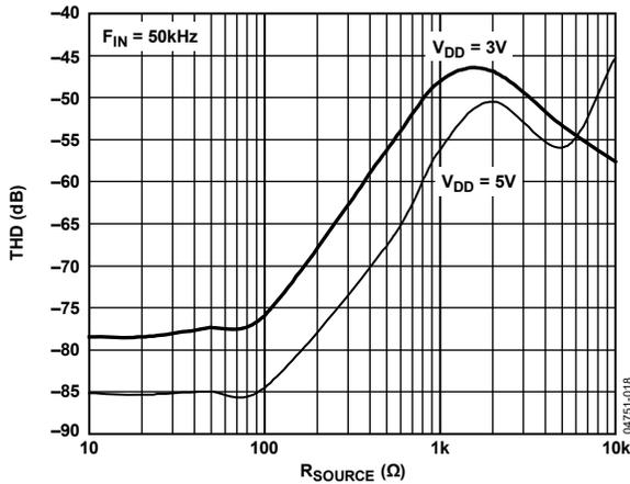
Figure 21. THD vs. Source Impedance in Single-Ended Mode
