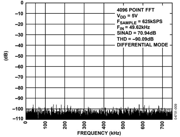
Figure 7. AD7938-6 FFT at V<sub>DD</sub> = 5 V
