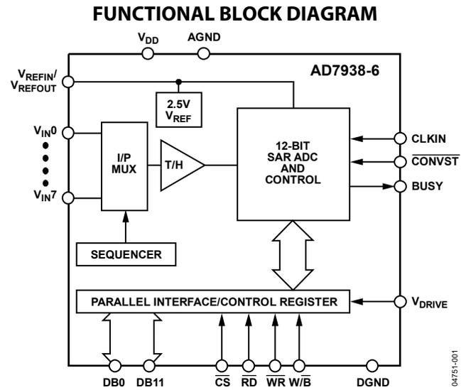
control register allows the user to set up different operating conditions, including analog input range and configuration, output coding, power management, and channel sequencing.
