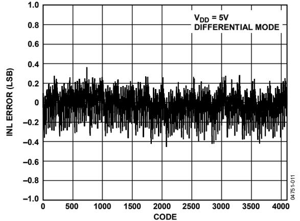
Figure 9. AD7938-6 Typical INL at V<sub>DD</sub> = 5 V
