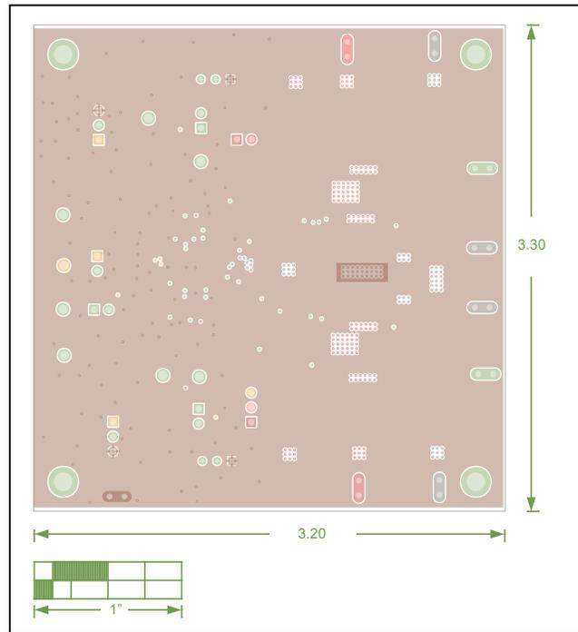
Figure 4. MAX20097 EV Kit PCB Layout—Inner Layer 1
