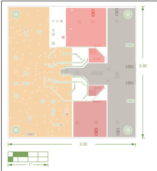
Figure 5. MAX20097 EV Kit PCB Layout—Inner Layer 2
