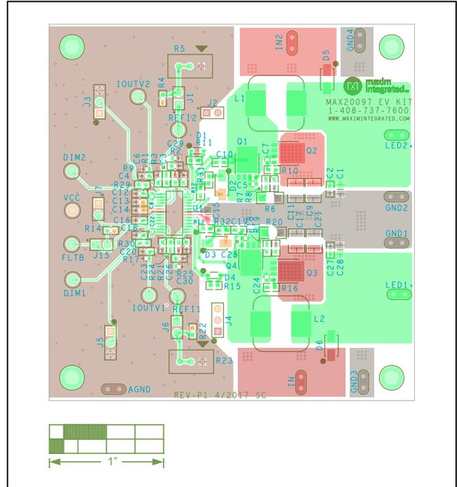
Figure 3. MAX20097 EV Kit PCB Layout—Top Layer
