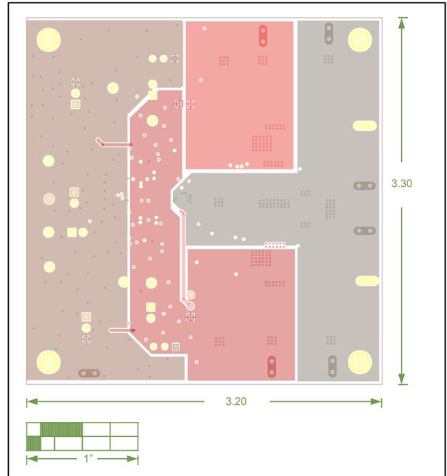
Figure 6. MAX20097 EV Kit PCB Layout—Bottom Layer
