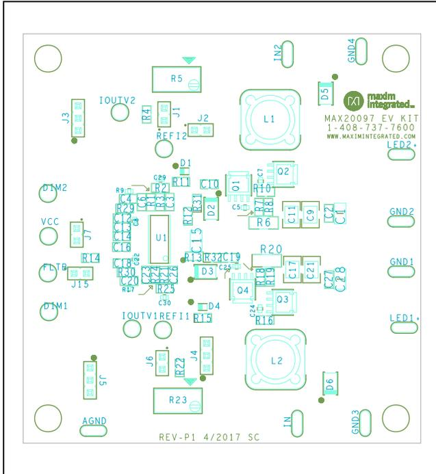
Figure 2. MAX20097 EV Kit Component Placement Guide—Component Side
