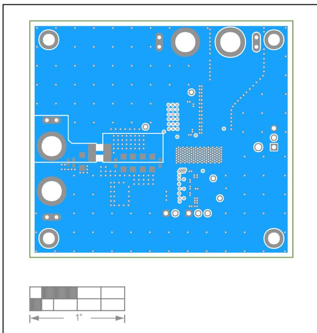
Figure 5. MAXM17536 5V Output EV Kit PCB Layout—Layer 4
