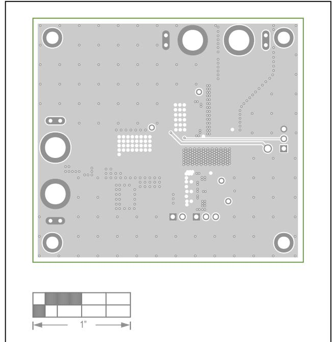
Figure 3. MAXM17536 5V Output EV Kit PCB Layout—Layer 2
