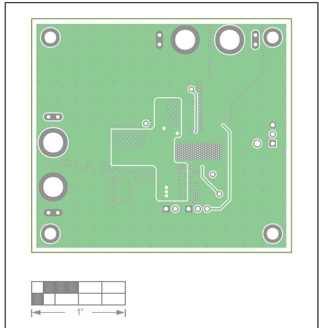
Figure 4. MAXM17536 5V Output EV Kit PCB Layout—Layer 3
