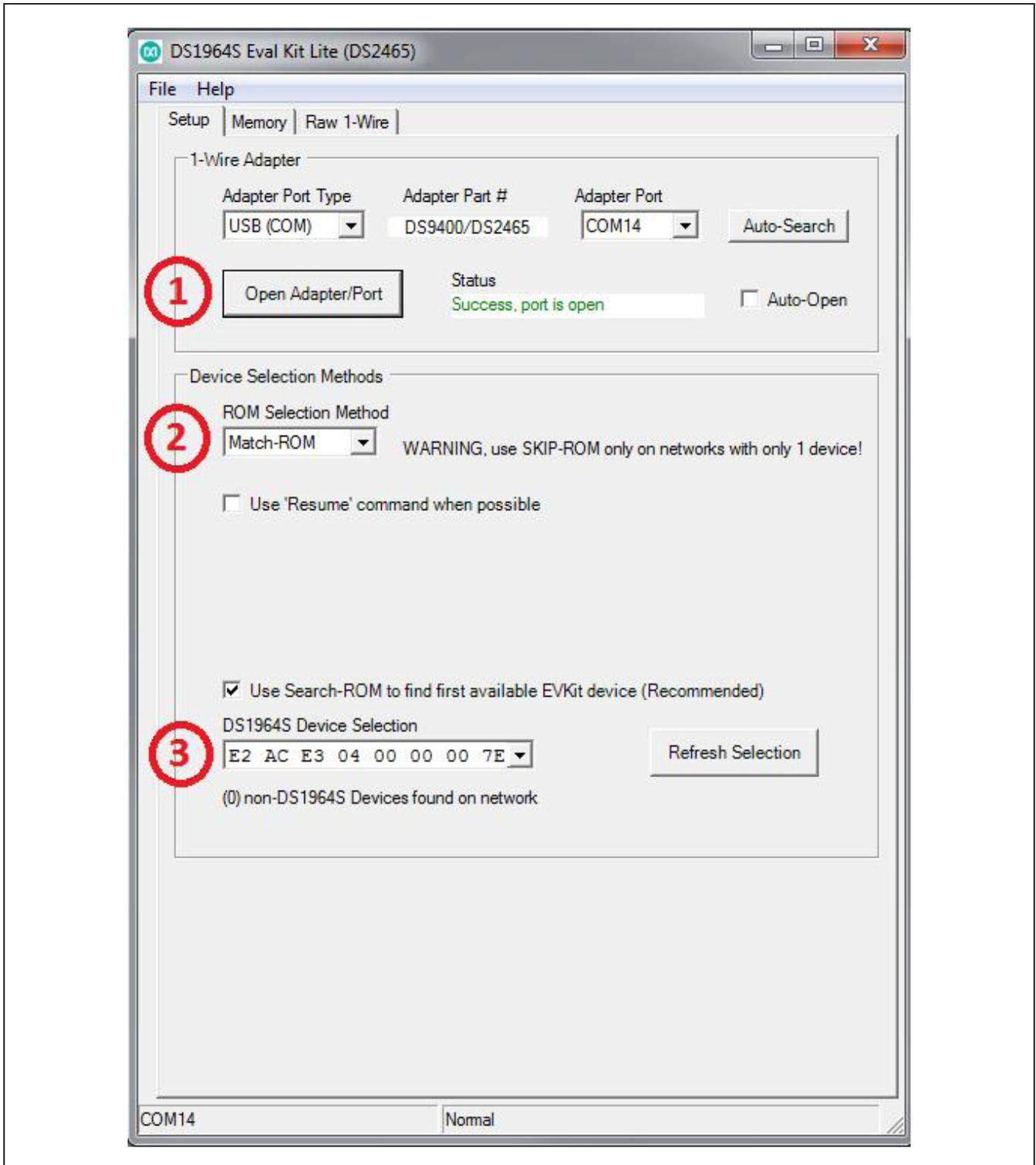
Figure 2. Evaluation Software: Main Window Setup Tab
