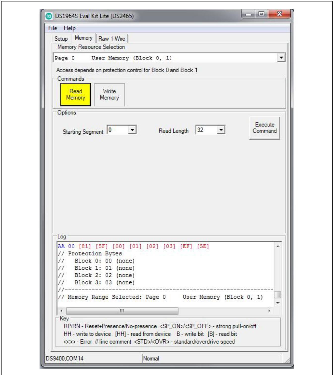
Figure 3. Evaluation Software: Main Window Memory Tab
