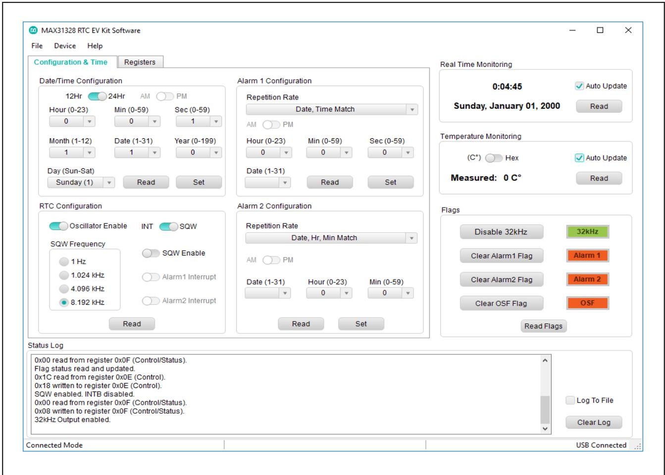
Figure 2. MAX31328 RTC Shield Software—Configuration & Time Page
