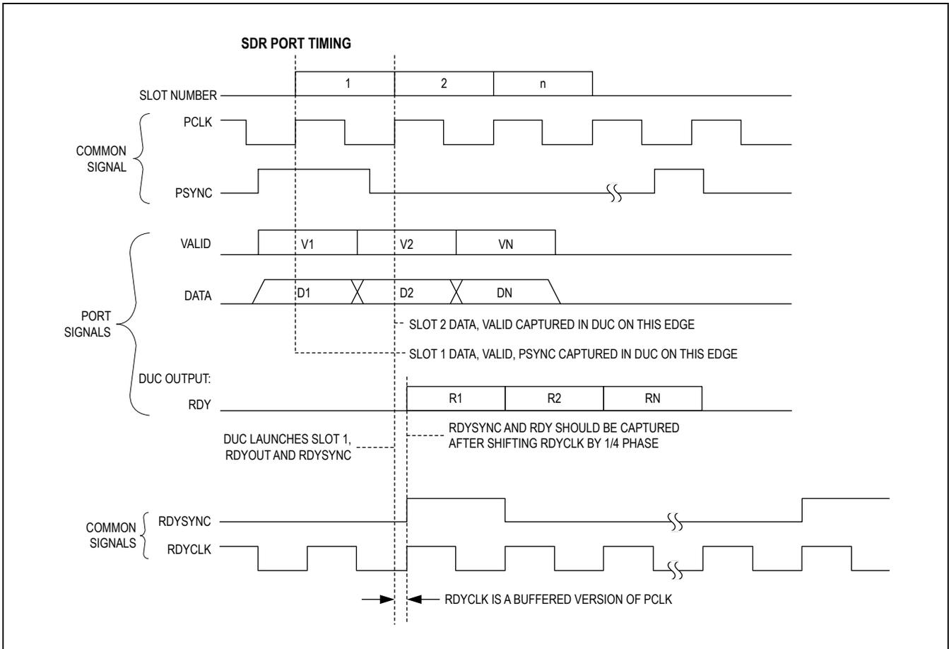
Figure 7. Example of Port Timing Diagram (SDR)
