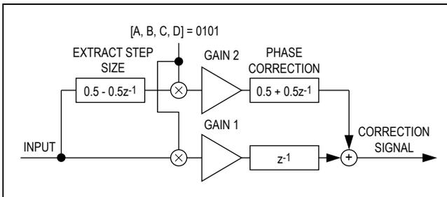
Figure 13. DAC Interleaving Error Compensation Block Diagram
