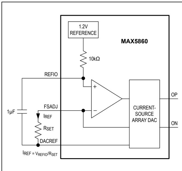
Figure 2. Reference System Architecture
