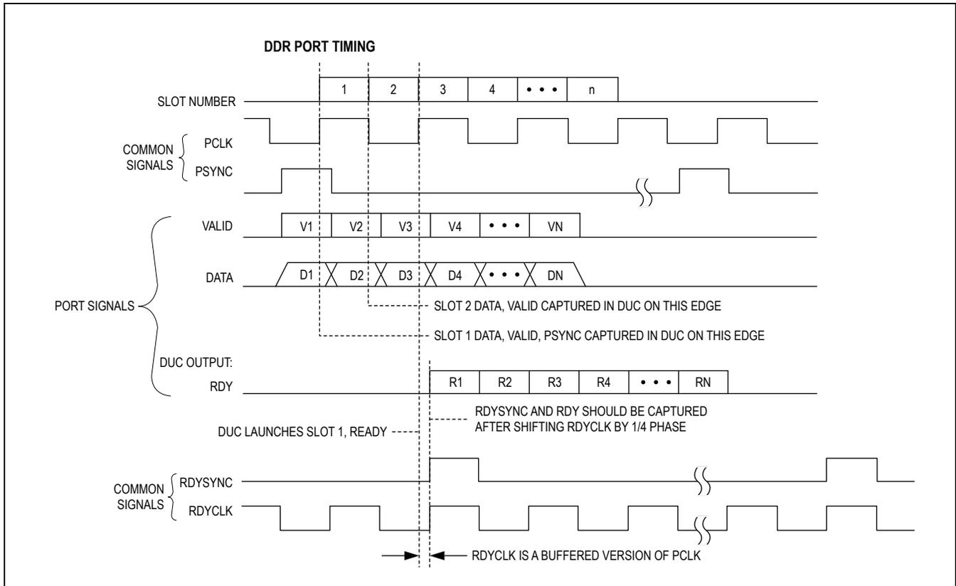
Figure 8. Example of Port Timing Diagram (DDR)
