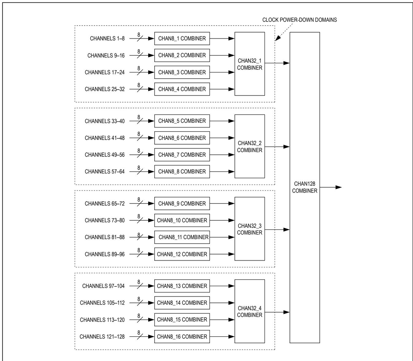
Figure 27. Channel and Block Combiner Numbering Reference
