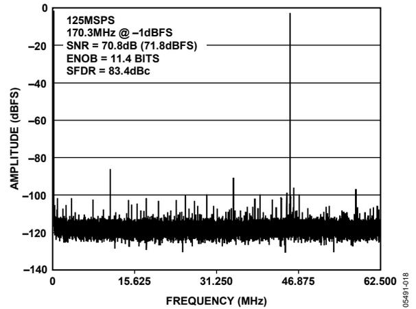
Figure 17. AD9246-125 Single-Tone FFT with  $f_{IN} = 170.3$  MHz
