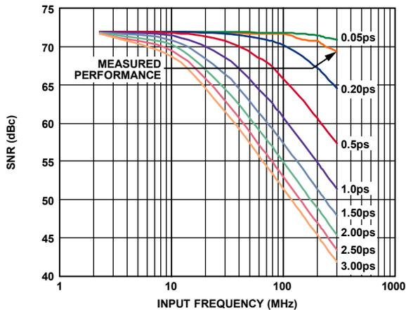
Figure 51. SNR vs. Input Frequency and Jitter
