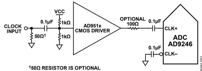
Figure 50. Single-Ended 3.3 V CMOS Sample Clock
