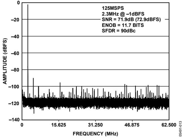
Figure 12. AD9246-125 Single-Tone FFT with  $f_{IN} = 2.3$  MHz
