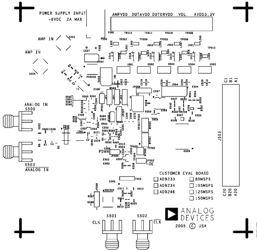
Figure 69. Evaluation Board Layout, Silkscreen Primary Side
