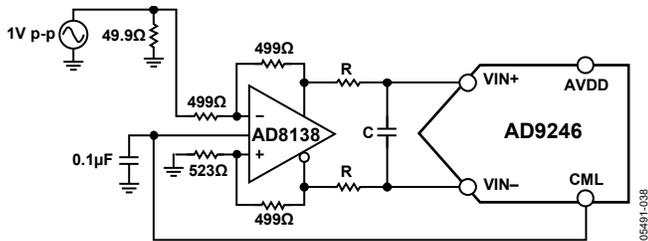
Figure 37. Differential Input Configuration Using the AD8138
