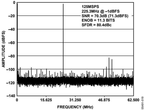
Figure 18. AD9246-125 Single-Tone FFT with  $f_{IN} = 225.3$  MHz
