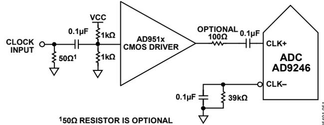
Figure 49. Single-Ended 1.8 V CMOS Sample Clock
