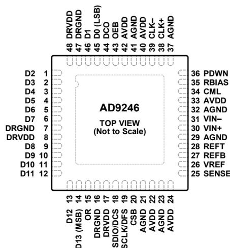
Figure 3. Pin Configuration
