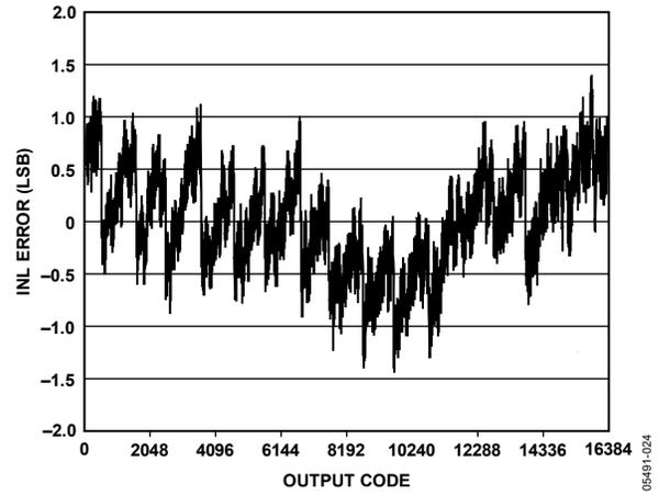
Figure 34. AD9246 INL with  $f_{IN} = 10.3$  MHz
