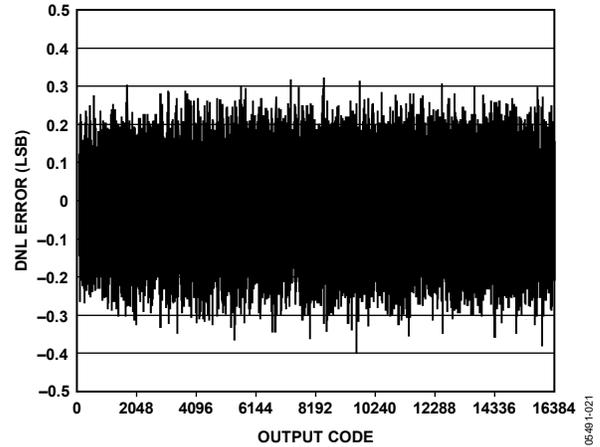
Figure 35. AD9246 DNL with  $f_{IN} = 10.3$  MHz
