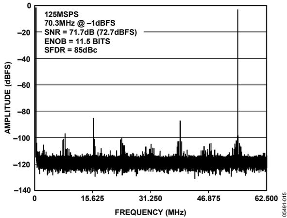
Figure 14. AD9246-125 Single-Tone FFT with  $f_{IN} = 70.3$  MHz
