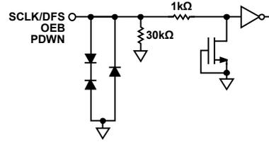
Figure 8. Equivalent SCLK/DFS, OEB, PDWN Input Circuit
