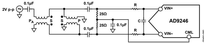
Figure 40. Differential Double Balun Input Configuration
