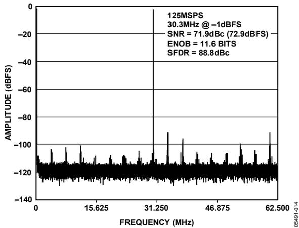
Figure 13. AD9246-125 Single-Tone FFT with  $f_{IN} = 30.3$  MHz
