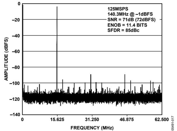
Figure 16. AD9246-125 Single-Tone FFT with  $f_{IN} = 140.3$  MHz
