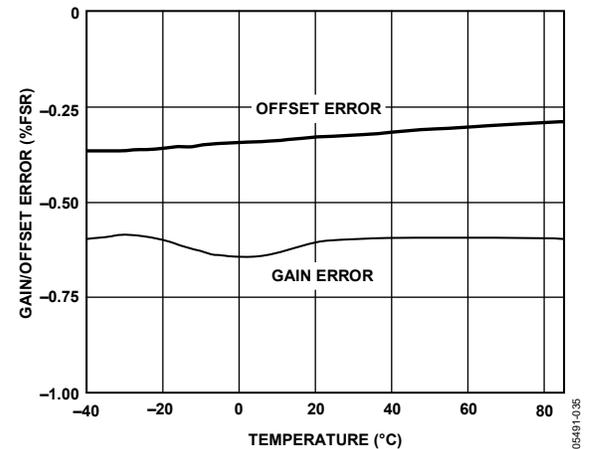
Figure 23. AD9246 Gain and Offset vs. Temperature
