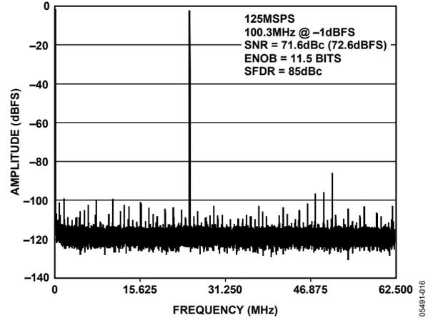
Figure 15. AD9246-125 Single-Tone FFT with  $f_{IN} = 100.3$  MHz
