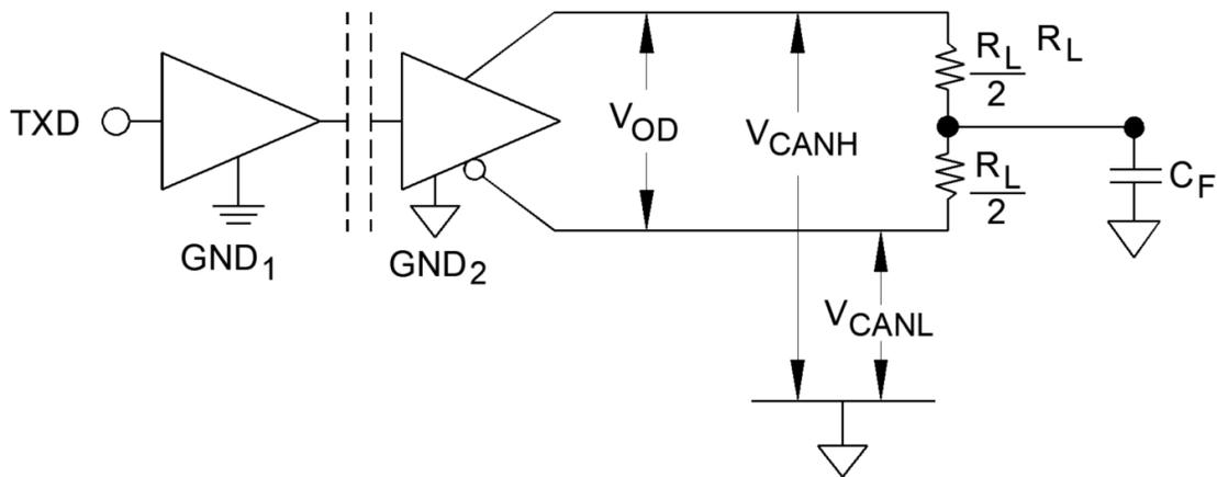
FIGURE 4. Driver voltage measurement.
