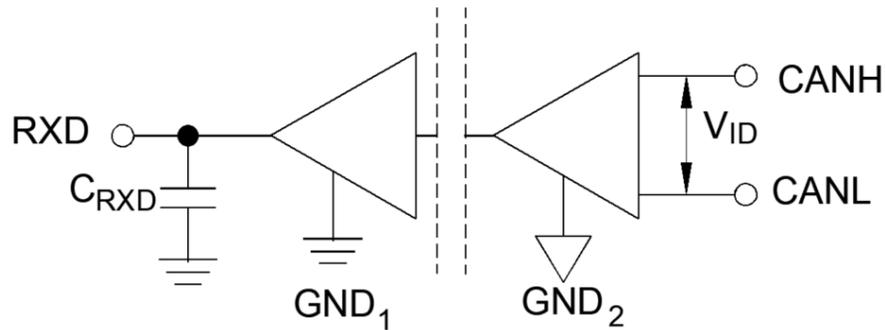
FIGURE 5. Receiver voltage measurement.
