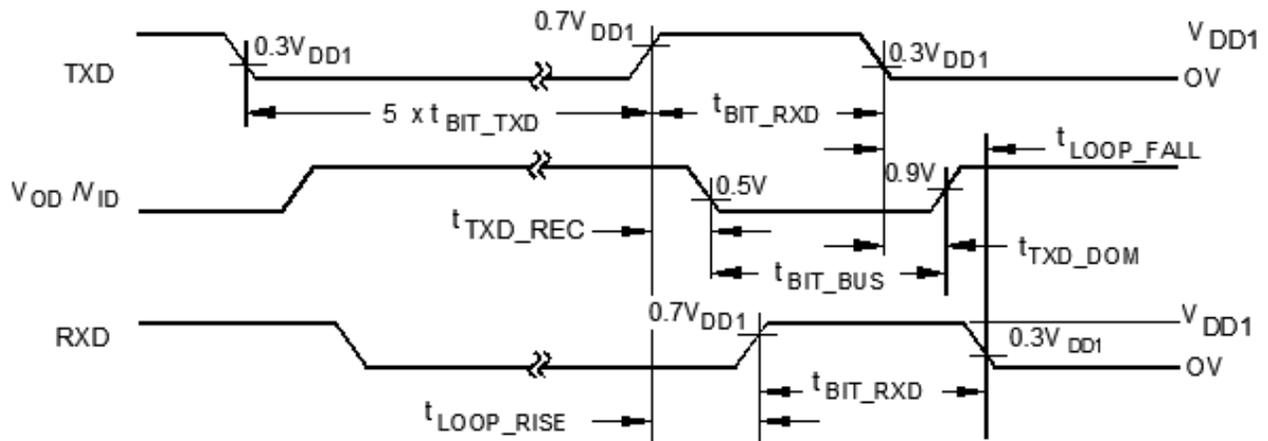
FIGURE 6. Transceiver timing diagram.
