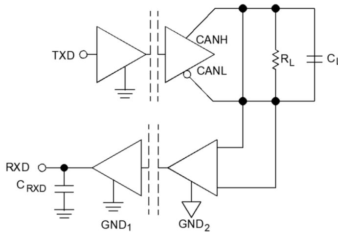
FIGURE 8. Switching characteristics measurements.
